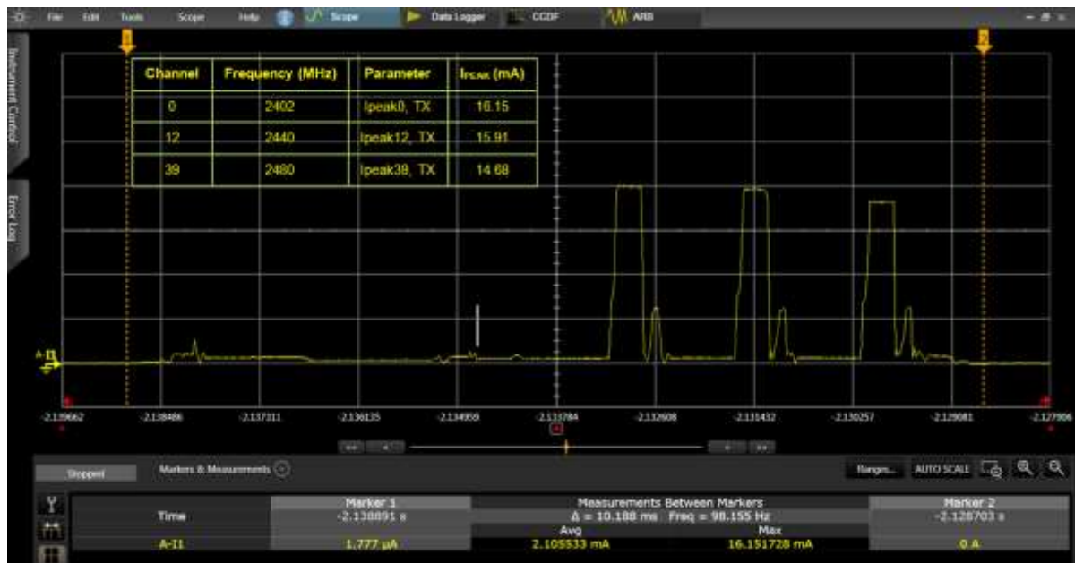
Figure 23: Current consumption for Advertisement frame
