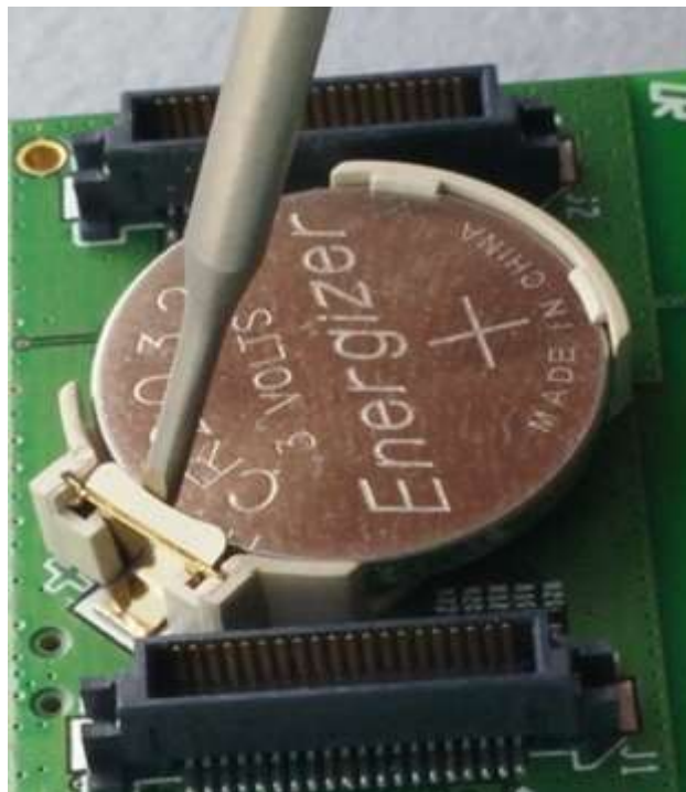
Figure 28: Recommended way of removing the coin cell battery from the battery holder
