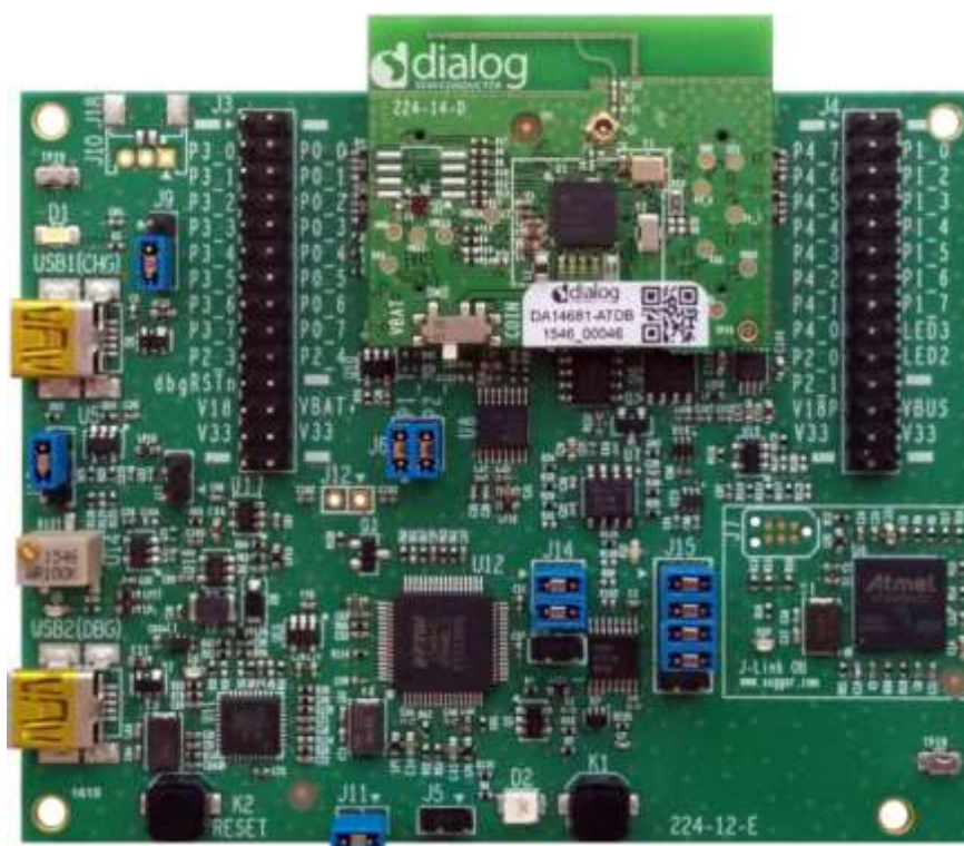
Figure 13: Jumper's placement for Full UART functionality
