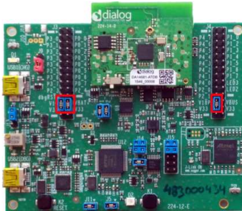
Figure 36 Shorting jumpers for lower VBAT
