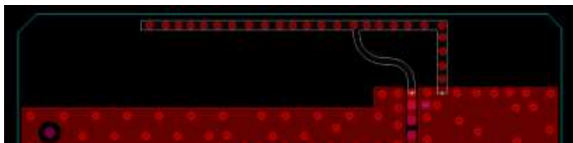
Figure 15: Printed Inverted F Antenna geometry
