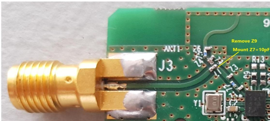
Figure 9: Modifications Required for Performing RF Measurements
