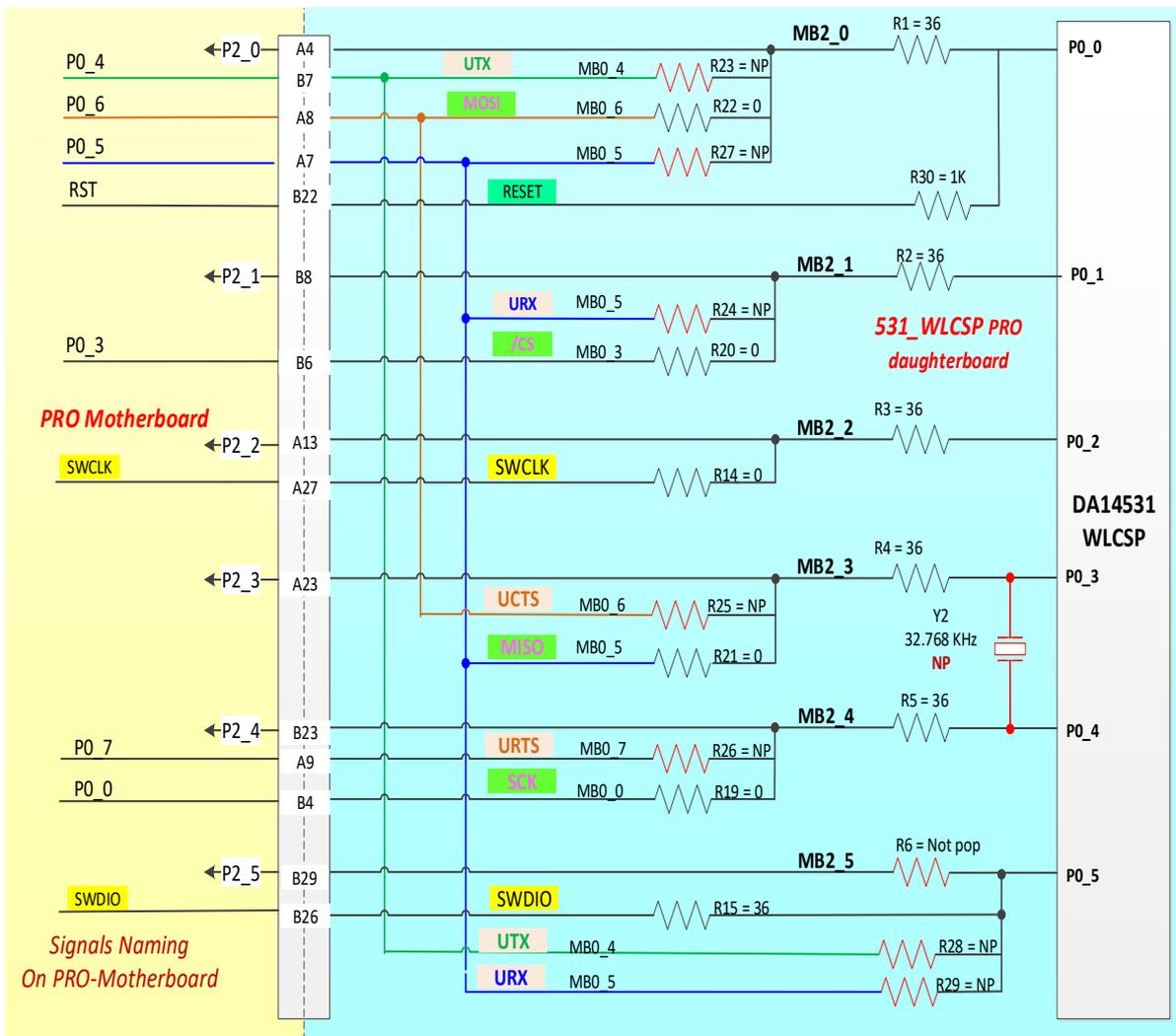
**Figure 65: System Configuration for DA14531 DK PRO with a DA14531 WLCSP17 PRO-DB (Default)**
