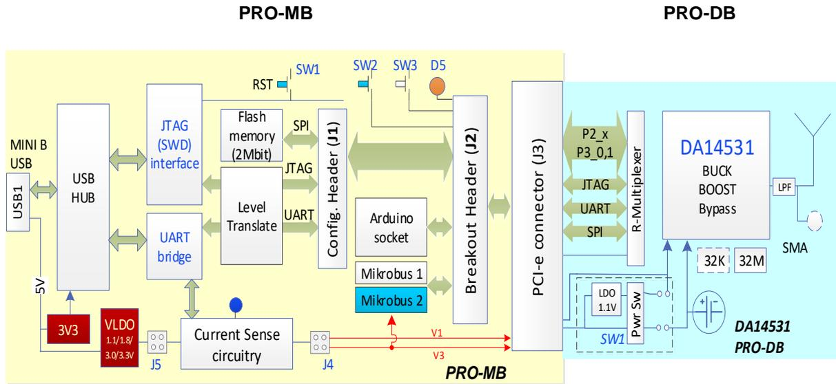
Figure 2: Block Diagram of the DA14531 DK PRO Hardware Platform
