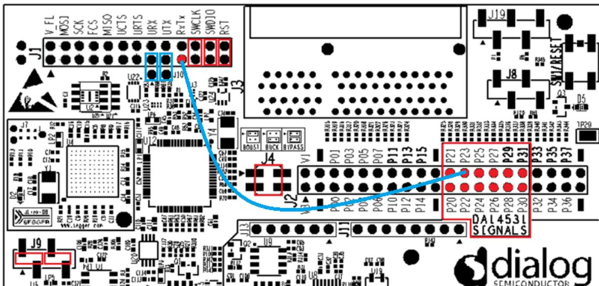
**Figure 24: Single-wire UART for DA14531 WLCSP17 PRO-DB**
