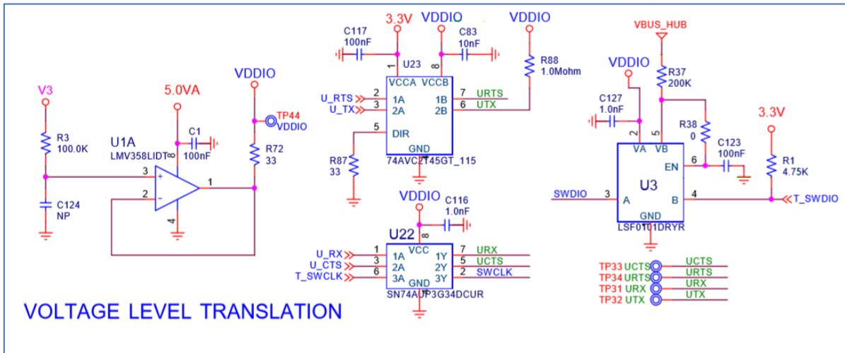
Figure 15: Voltage Translator Circuitry of DA14531 PRO-MB
