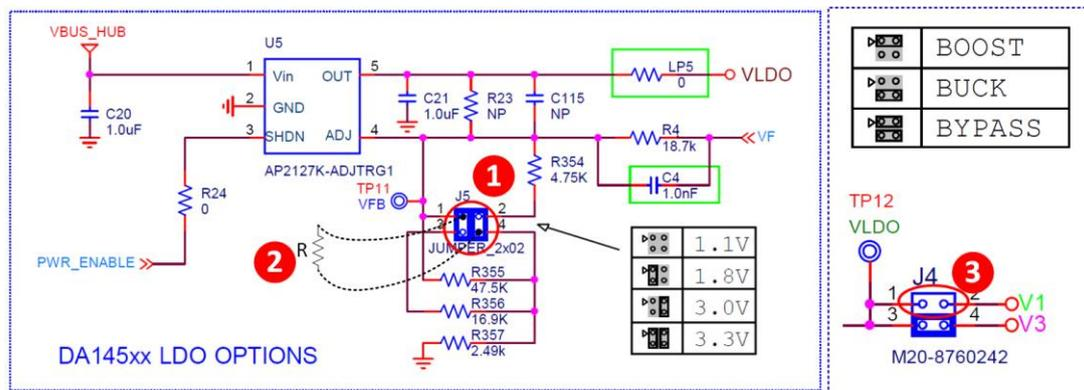
Figure 75: Configuring VLDO for 1.5 V Boost Operation
