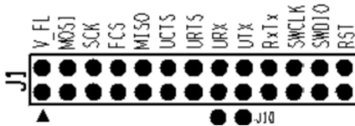
Figure 19: J1, Configuration Header on DA14531 PRO-MB
