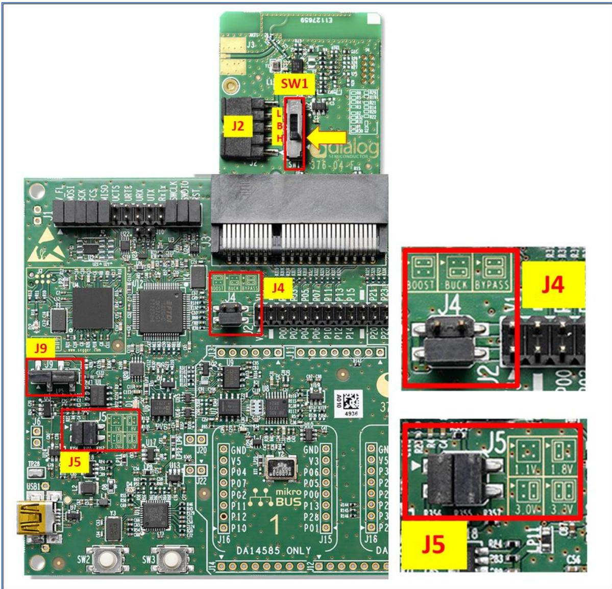
Figure 30: DA14531 PRO-DB Configuration and DA14531 PRO-MB Jumpers
