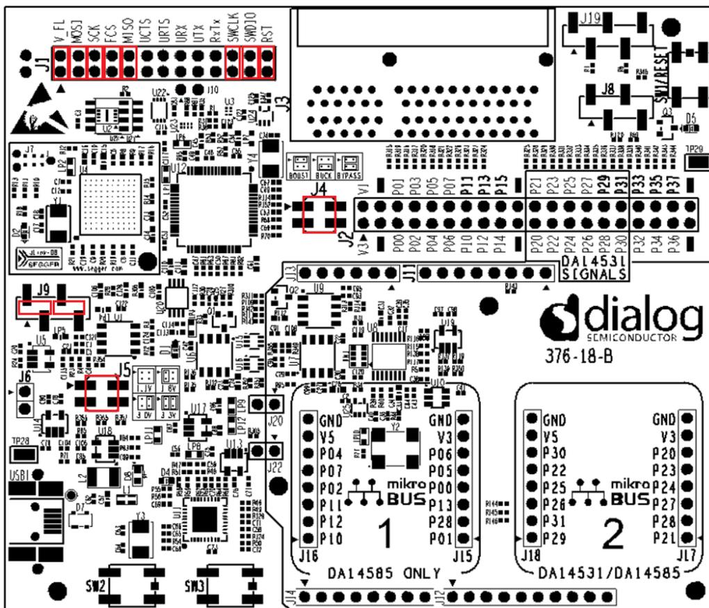
Figure 68: Jumper Settings for PRO-MB (Marked in Red)
