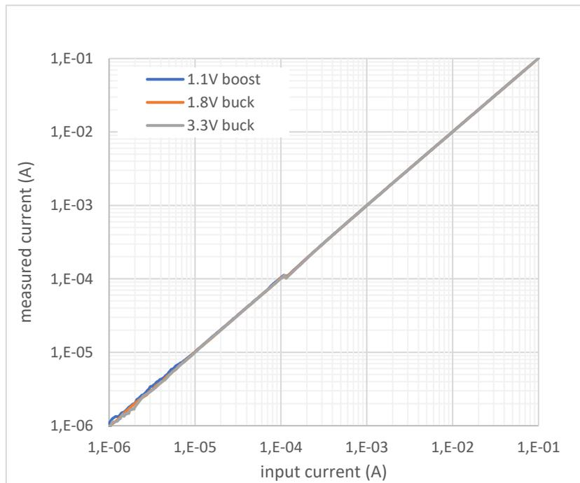
Figure 50: Current Measurement Circuit Response, Indicative Graph
