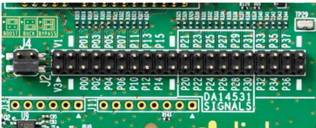
Figure 18: J2, Breakout Header of DA14531 PRO-MB
