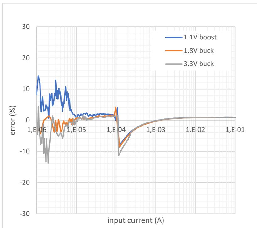
Figure 51: Current Measurement Circuit Inaccuracy, Indicative Graph
