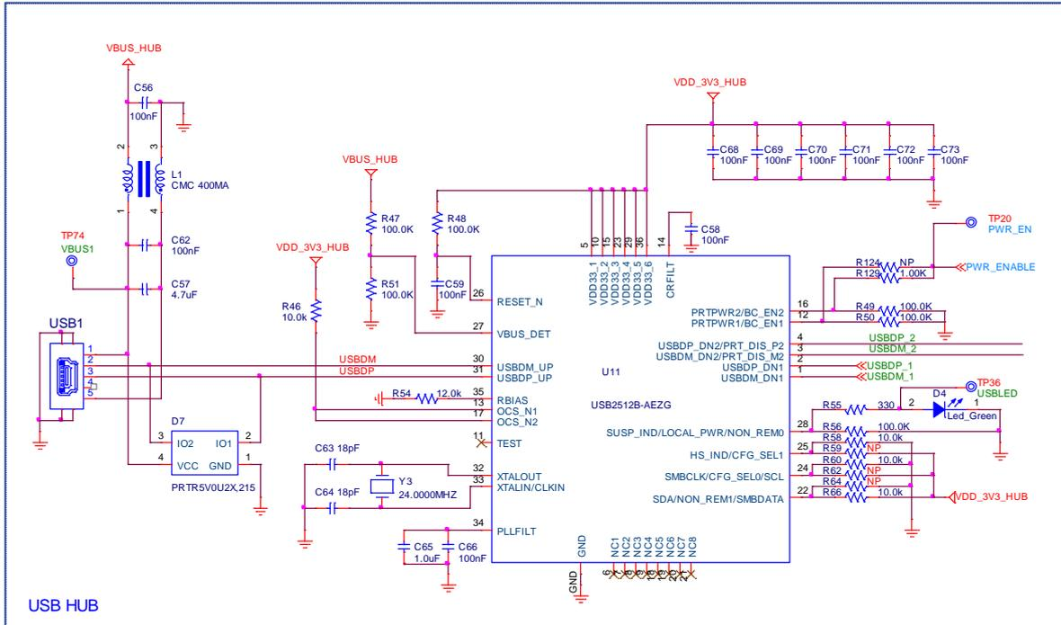
Figure 12: USB HUB Circuitry of DA14531 PRO-MB
