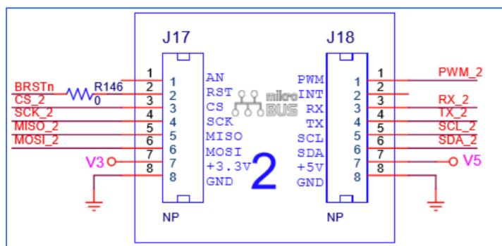
Figure 29: MikroBus 2 Circuit
