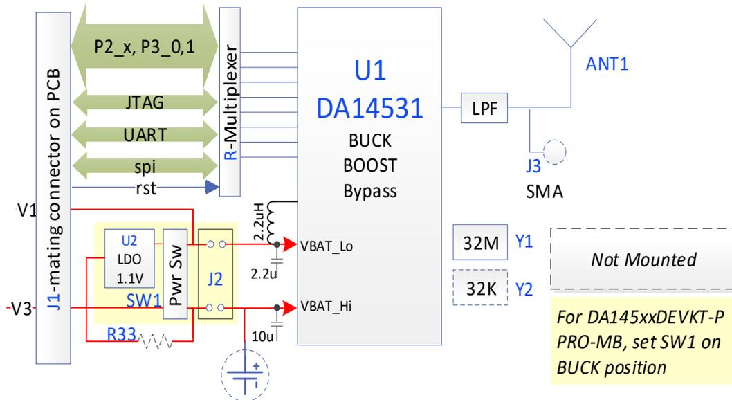
Figure 3: System Block Diagram of DA14531 PRO-DB
