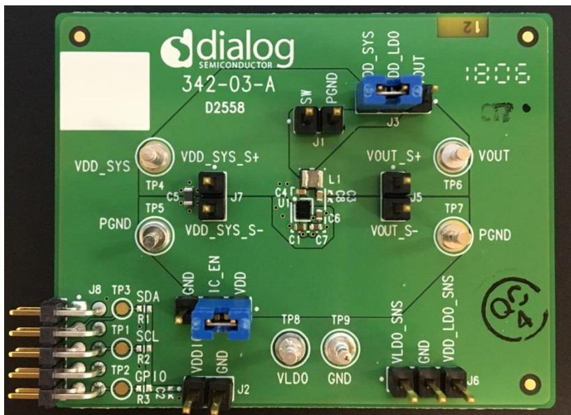
Figure 1: 342-03-A Evaluation Board Top View
