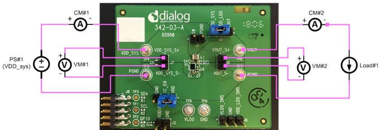
Figure 4: Recommended Setup for Buck Efficiency Measurement
