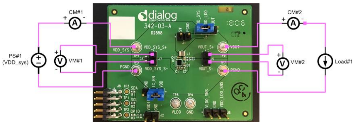
Figure 4: Recommended Setup for Buck Efficiency Measurement
