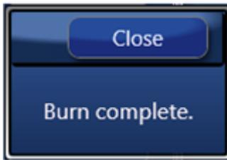
**Important:** Burning irreversibly converts ones to zeroes; it is possible to go back and burn an unburned bit or bits to zero; zeroes cannot be restored to ones. This allows revision of a burn under limited circumstances.
