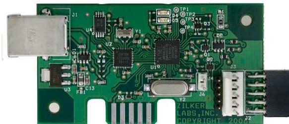
Figure 1. USB to SMBus Interface
