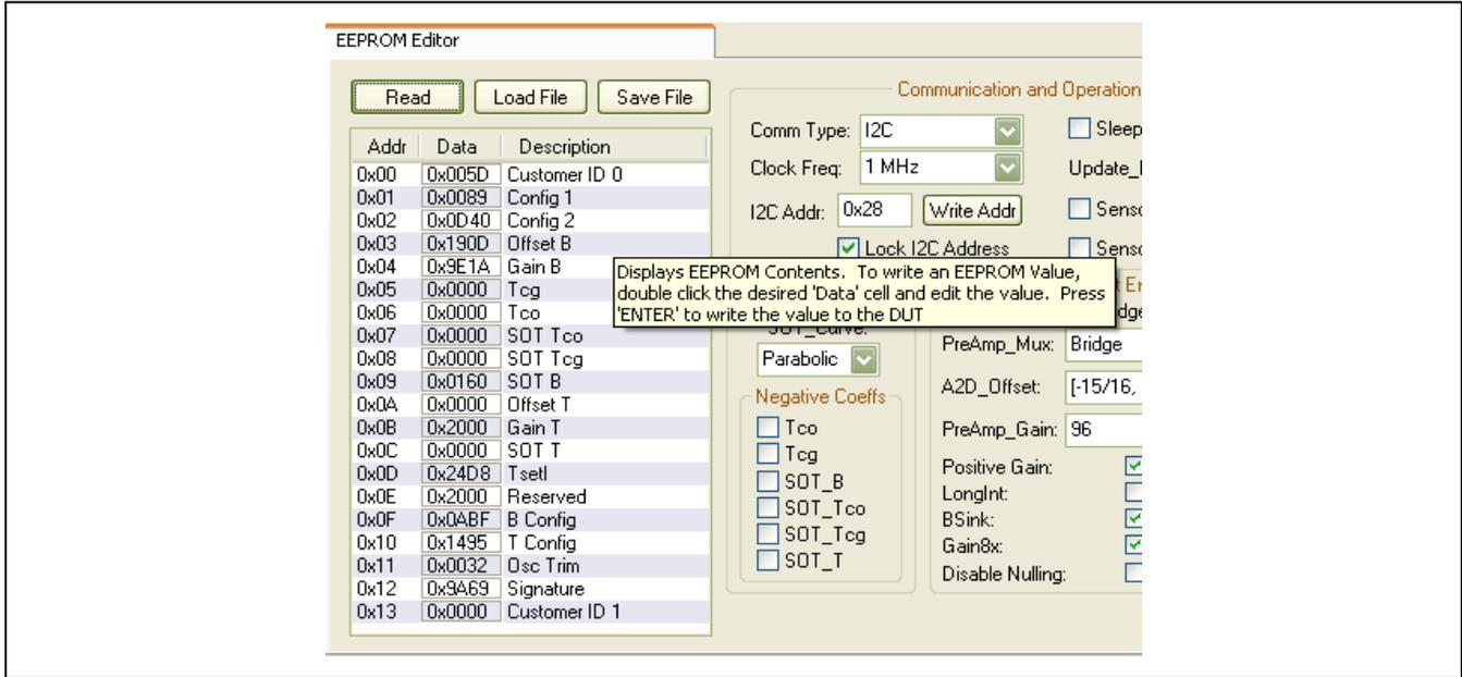
**Note:** EEPROM words 10<sub>HEX</sub>(T\_Config) and 11<sub>HEX</sub>(Osc Trim) are trimmed individually during IDT’s final test (For more details, see the ZSC31014 Rbic<sub>iLite</sub>™ Data Sheet). Important: Ensure that these words are not overwritten.
