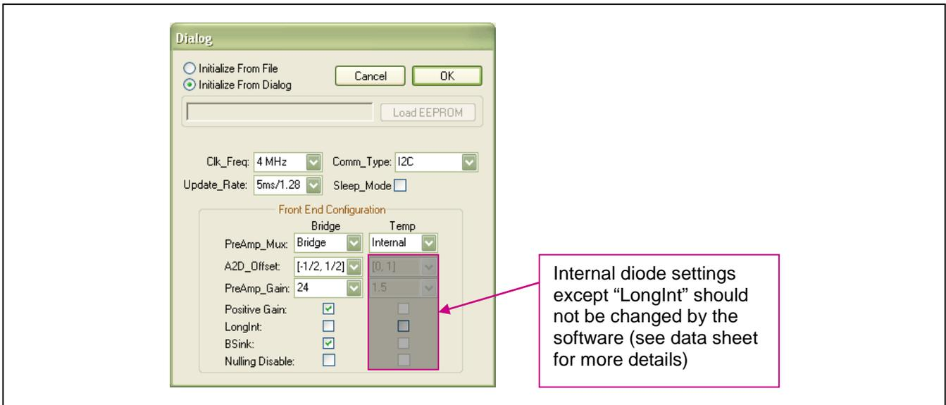
9. The next step is to start data collection. Normally this would be done with a real bridge attached to the ZSC31014 on a remote board in a controlled chamber. Instead, this dry run calibration uses the artificial bridge inputs controlled by the on-board DAC. The DAC is controlled by the “Artificial Stimulus” slider bar or its adjacent entry field at the top of the calibration window (see Figure 4.4).
