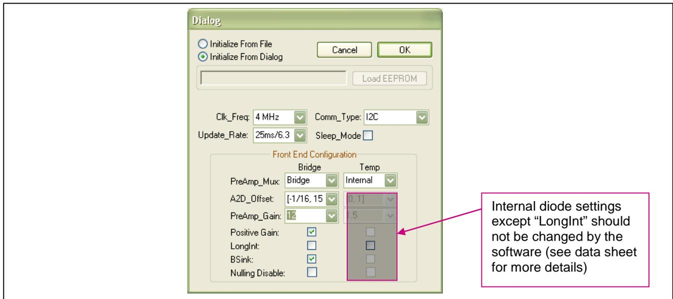
9. The next step is to start data collection. Normally this would be done with a real bridge attached to the ZSC31014 on a remote board in a controlled chamber. Instead, this dry run calibration uses the Sensor Replacement Board (SRB) as bridge inputs.
