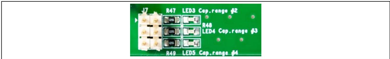
It is important to ensure that the output capacitor range selected on J7 matches the compensator selected for the ZSPM1025C. The compensator can be selected on DIP switch J5 on switches 5 through 8 (see Table 6.2).
