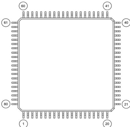
Note 1: If the Special Mark is to be printed, indicate the desired layout of the mark in the left figure. The layout will be duplicated technically as close as possible. Renesas lot number (6-digit or 7-digit) and Mask ROM number (3-digit) are always marked.
