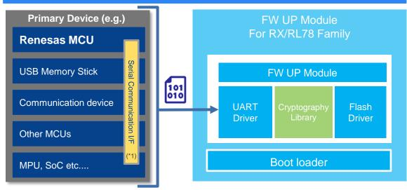
\*1: A serial communication sample (C-source) to communicate with its FW UP Module can also be provided if required.
