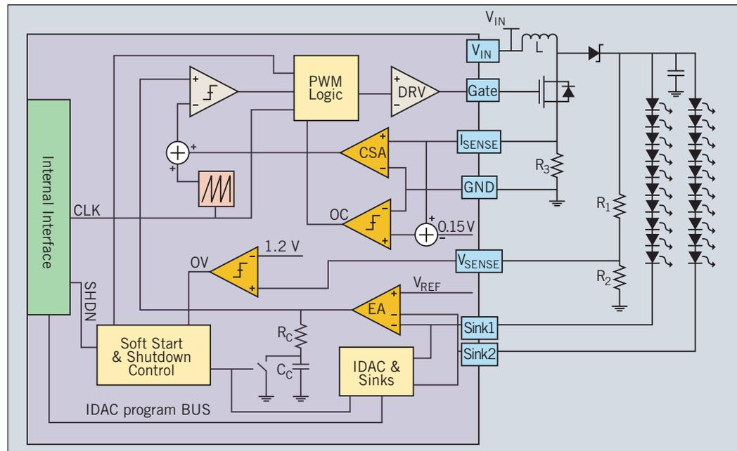
charging to the programmed output voltage using soft start. During soft-start, the BOOST5 limits the peak inductor current for the first 500  $\mu$ s. The voltage value in the output voltage register may be changed during soft-start.
