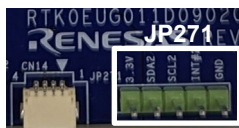
Figure 4-2 Connector for SMBus Slave Interface
