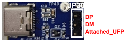
Figure 4-1 Connector for USB2.0 based peripheral debugging
