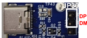
Figure 3-2 Connector for Power Bank mode setting
