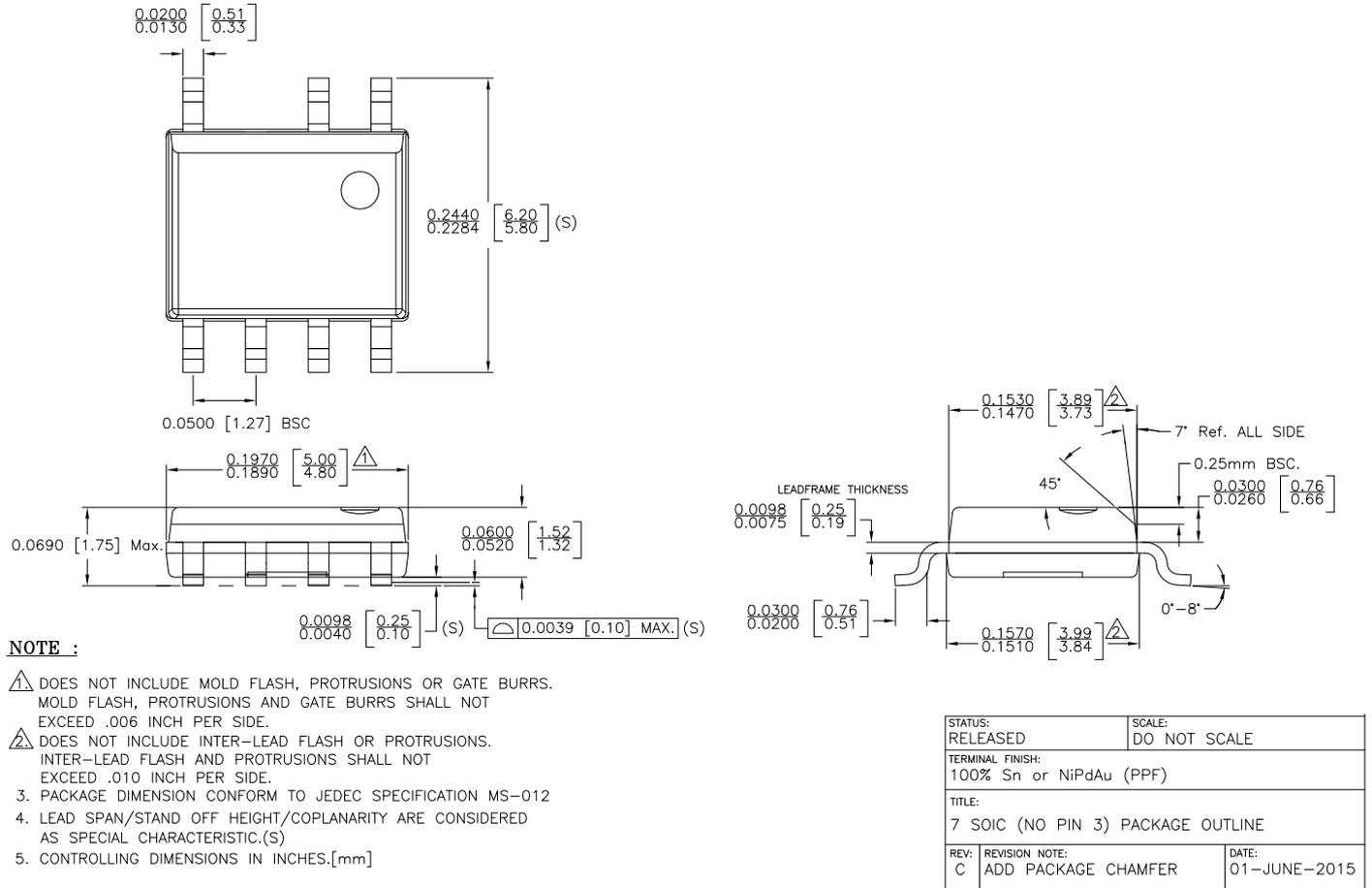
Figure 6.1 : 7-Lead SOIC Package Outline Drawing
