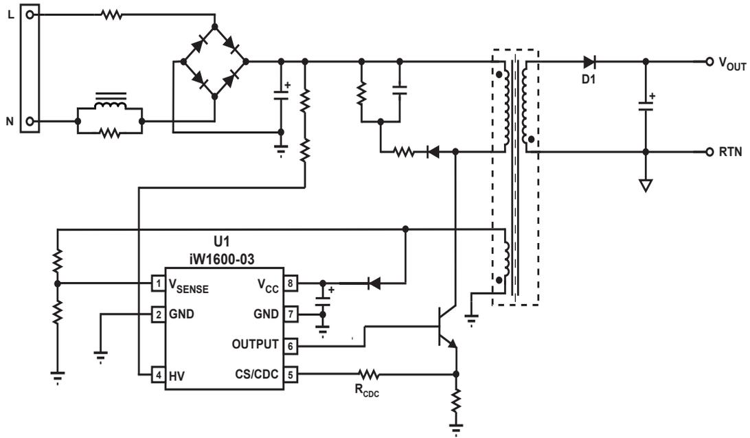
Figure 3.1: iW1600-03 Typical Application Circuit
