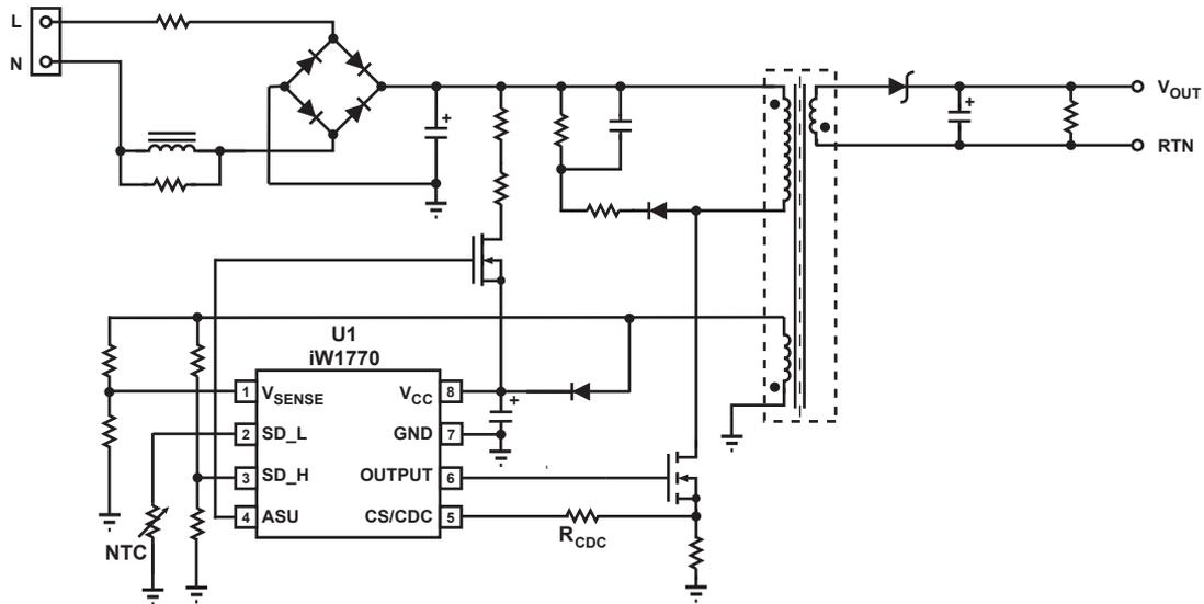
**Figure 3.1 : iW1770 Typical Application Circuit
