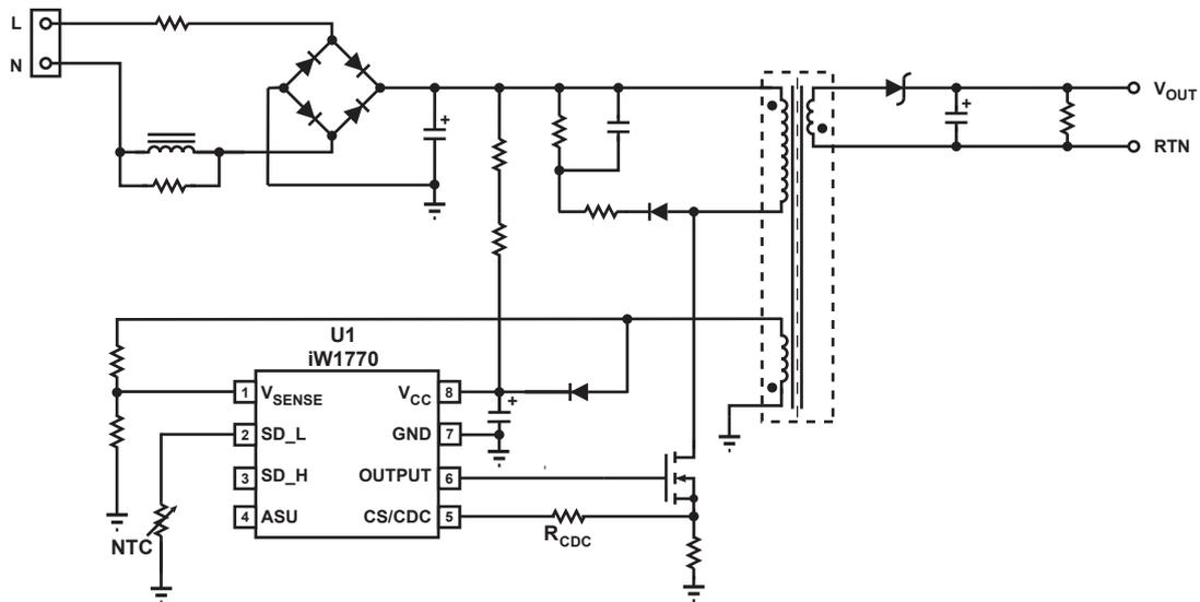
**Figure 3.2 : iW1770 Typical Application Circuit
