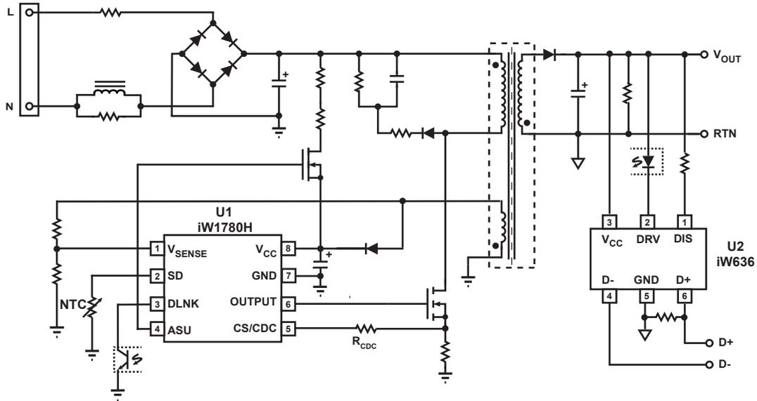
Figure 3.1 : iW1780H Typical Application Circuit for Multi-Level Output Voltage and Current (Using iW636 as Secondary-Side Controller for QC3.0. Achieving < 10mW No-Load Power Consumption in Typical 15W Design)
