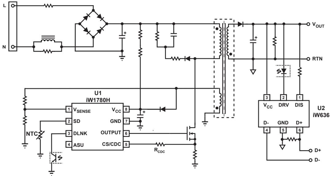
Figure 3.3 : iW1780H Typical Low Cost Application Circuit for Multi-Level Output Voltage and Current (Using iW636 as Secondary-Side Controller for QC3.0. Achieving < 50mW No-Load Power Consumption Without Using Active Start-up Device)
