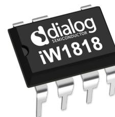
**Off-Line Digital Green-Mode Quasi-Resonant PWM Controller Integrated with Power BJT**
