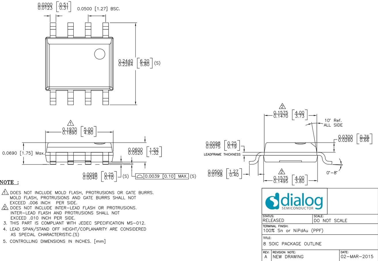
Figure 6.1 : Physical Dimensions of 8-Pin SOIC Package
