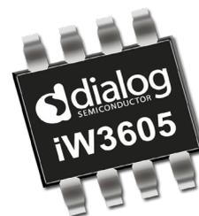
AC/DC Digital Power Controller for Bleederless Single-Stage High Power Factor Dimmable LED Drivers
