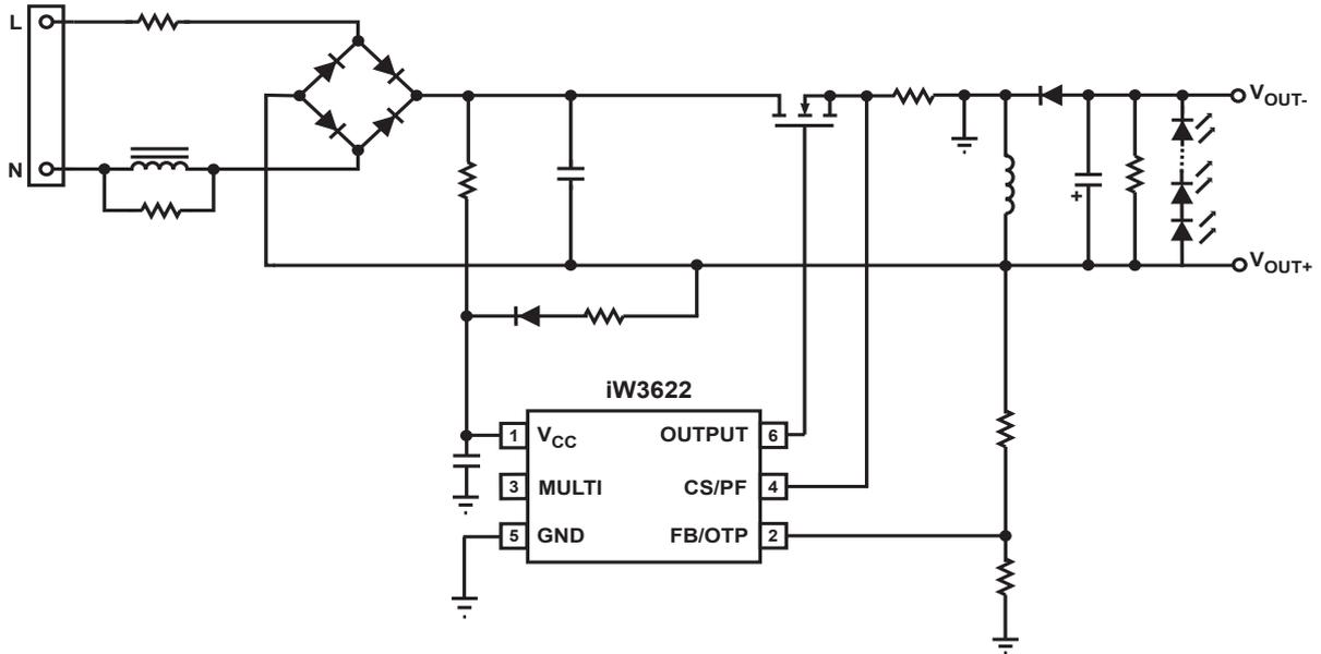
Figure 3.1 : iW3622 Typical Application Circuit (Non-Isolated Buck-Boost Application)
