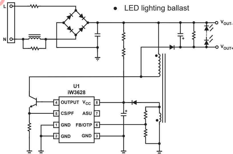
Figure 3.1: iW3628 Typical Application Circuit (Non-Isolated Application)
