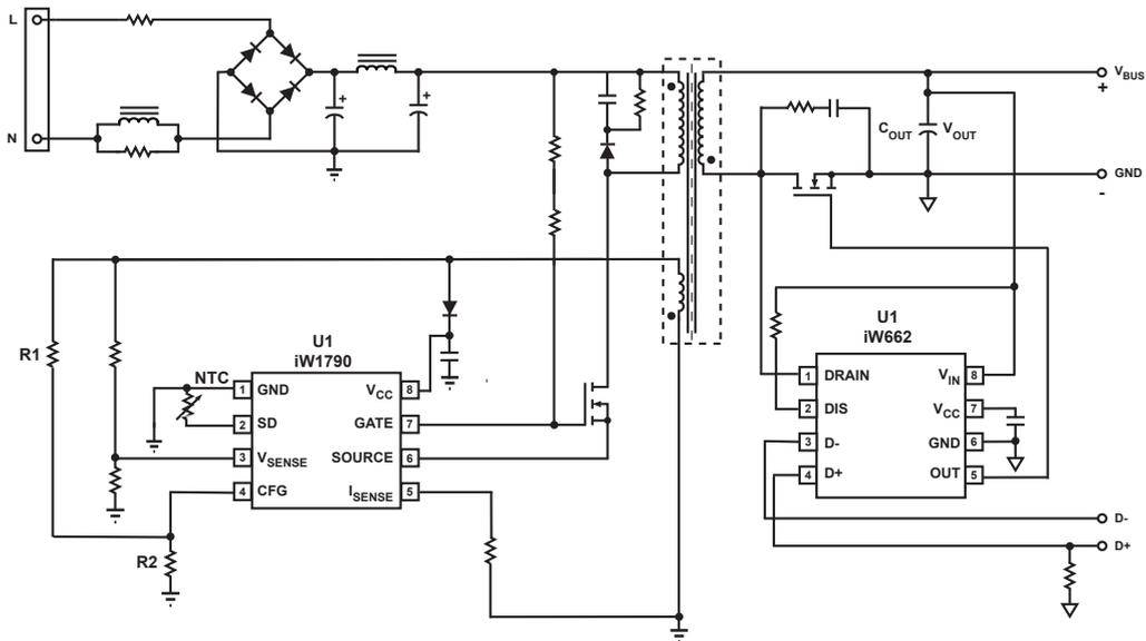
**Figure 3.1 : iW662 18W/24W Typical Application Circuit for Multi-Level Output Voltage and Current (Using iW1790 as Primary-Side Controller. Achieving < 20mW No-Load Power Consumption.)**
