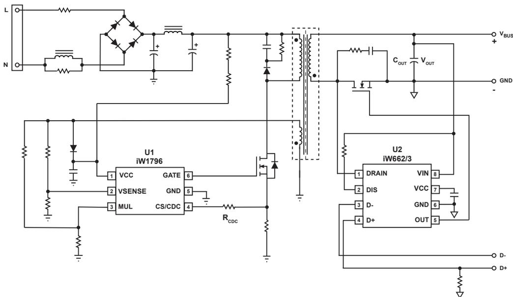
**Figure 3.2 : iW1796 Typical Application Circuit for Multi-Level Output Voltage and Current (Using iW662/3 as Secondary-Side Controller for Rapid Charge Protocols. Achieving < 75mW No-Load Power Consumption (with ample margin) in Typical 15W Design.)**
