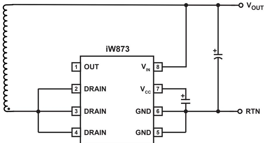
Figure 3.1 : iW873 Typical Application Circuit
