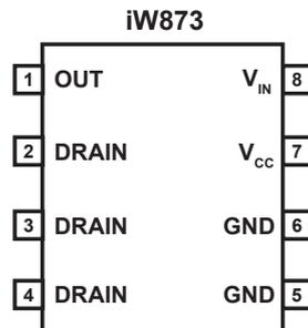
Figure 4.1 : 8-Lead SOIC Package
