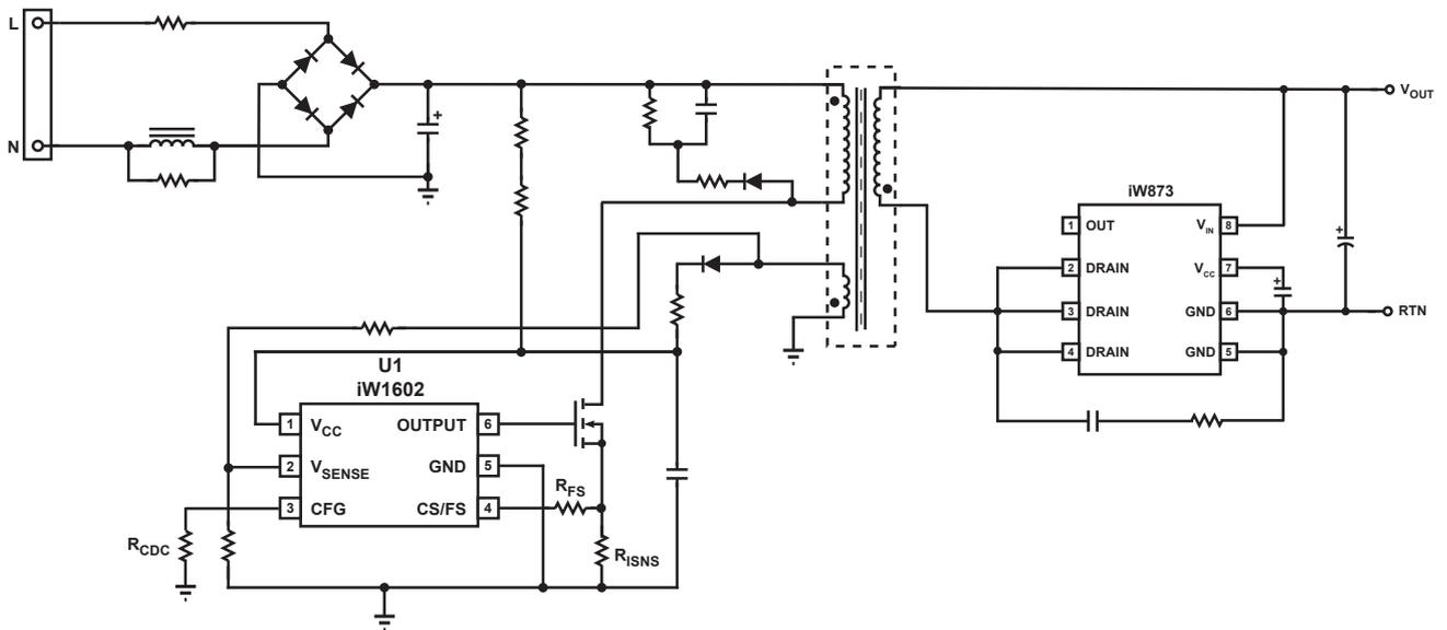
**Figure 3.2 : iW873-00 Typical Application Circuit (Using iW1602 as Primary-Side Controller)**
