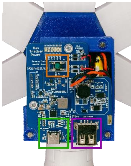
Figure 4. Sun Tracker Power Panel
