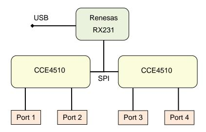
For demonstrating the functionality of the system, it can be controlled over USB using the USB IO-Link Device Tool software, which runs on a Windows PC.
