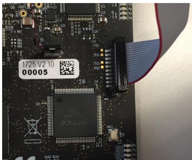
Figure 2-3: I-Jet Debugger connection
