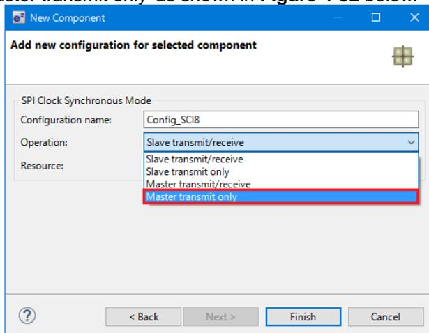
**Figure 4-32 Select Operation – Master Transmit only**
