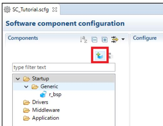
Figure 4-5 Add a Code Generator component (1)
