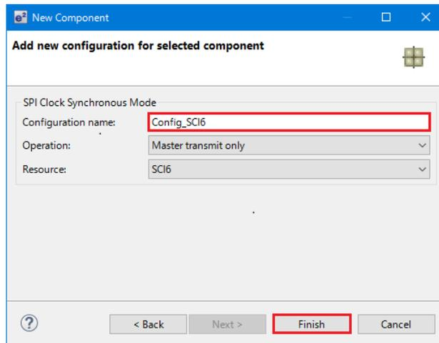
**Figure 4-34 Ensure Configuration name - Config\_SCI6**
