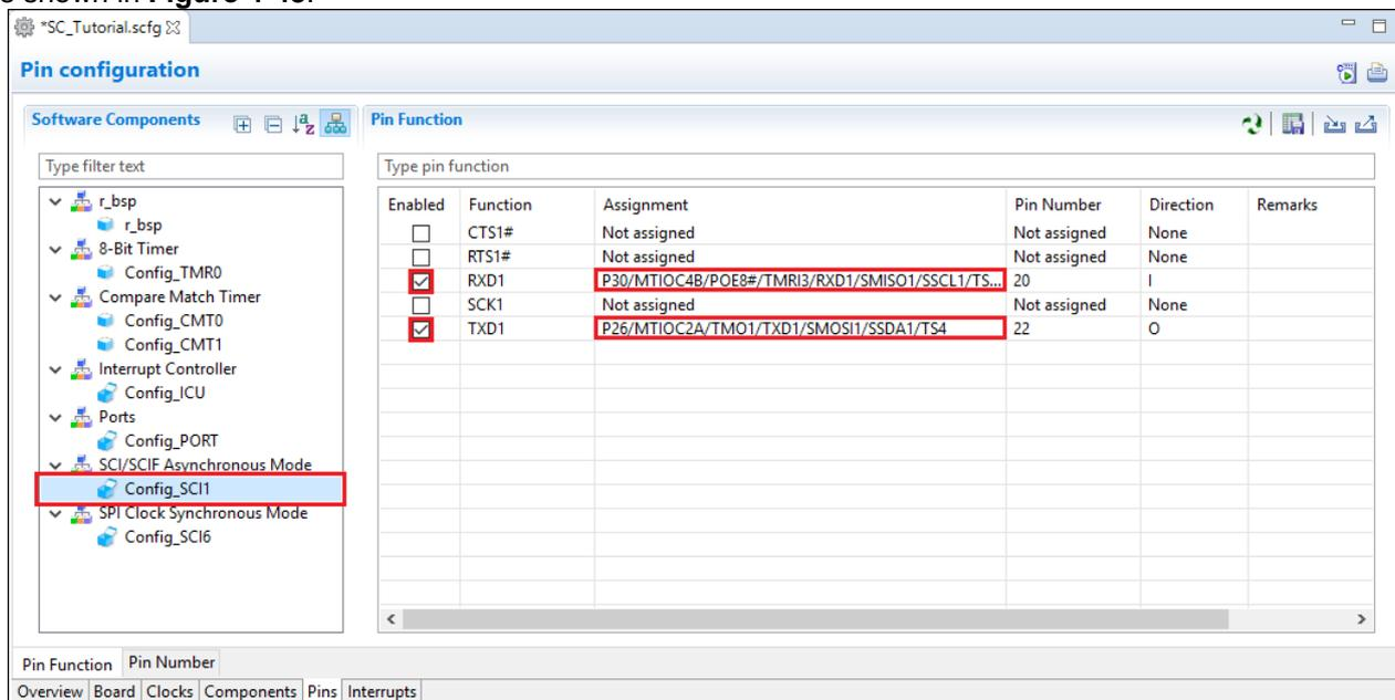
Figure 4-43 Configure pin assignment - Config\_SCI1
