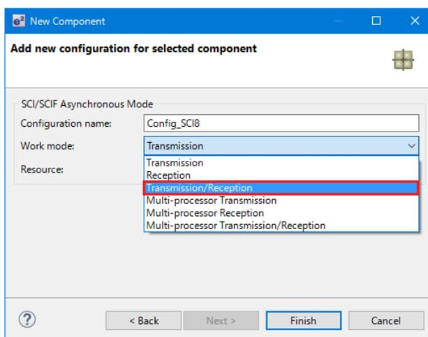
**Figure 4-27 Select Work mode – Transmission/Reception**
