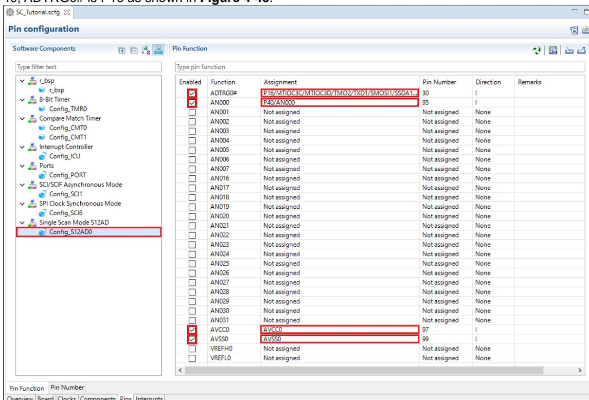
Figure 4-45 Configure pin assignment - Config\_S12AD0
