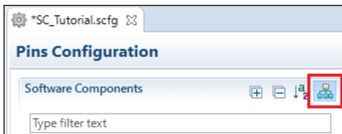
Figure 4-41 Change view to show by Software Components
