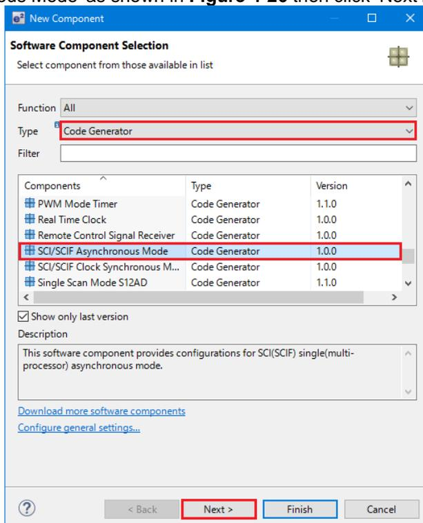
**Figure 4-26 Select SCI/SCIF Asynchronous Mode**
