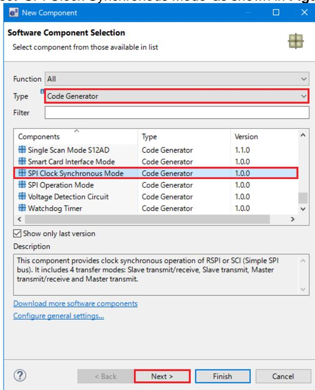
**Figure 4-31 Select SPI Clock Synchronous Mode**
