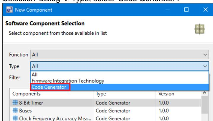
Figure 4-6 Add a Code Generator component (2)
