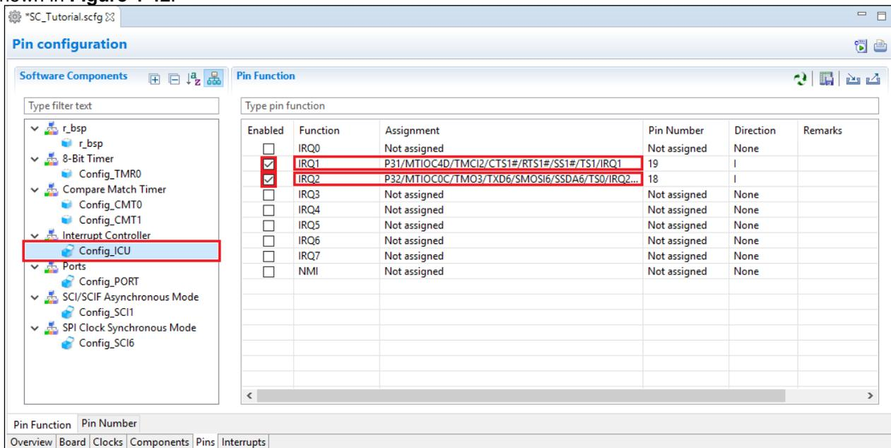
Figure 4-42 Configure pin assignment - Config\_ICU
