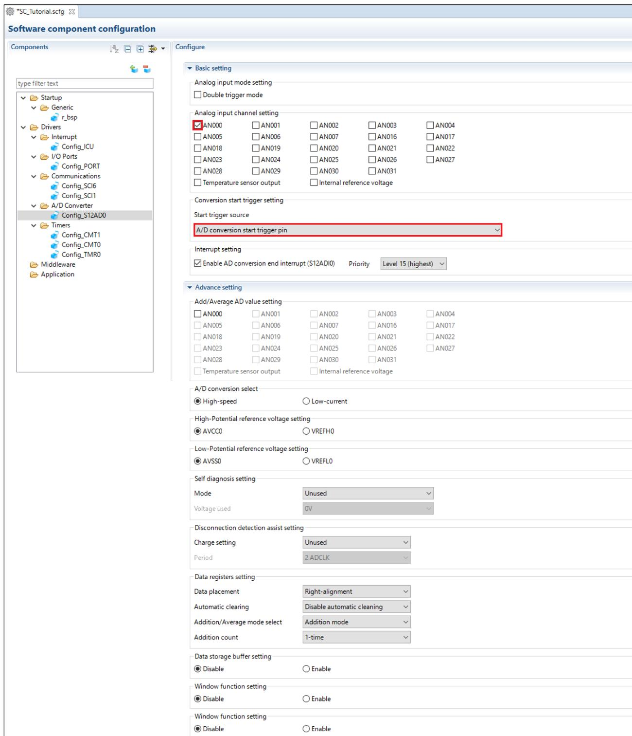
**Figure 4-38 Config\_S12AD0 setting (1)**
