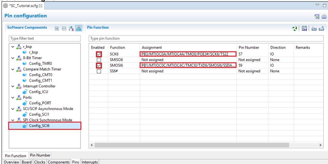
Figure 4-44 Configure pin assignment - Config\_SCI6
