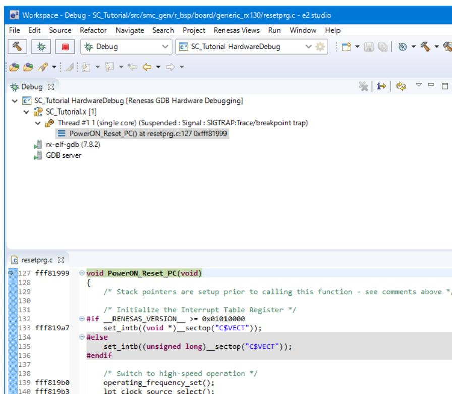
**Figure 6-4 Debugger start up screen**
