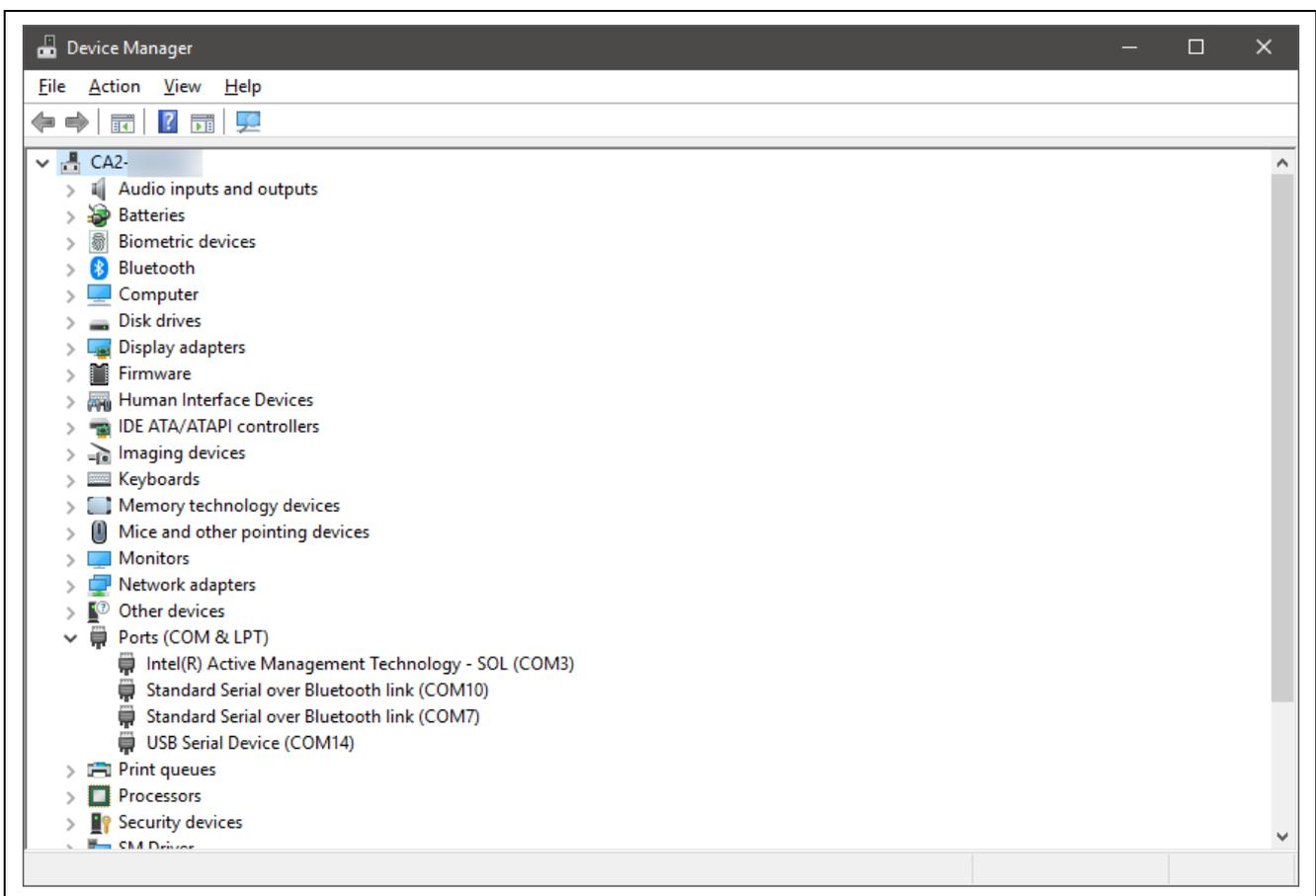
Figure 4. USB Serial Device in Windows Device Manager
