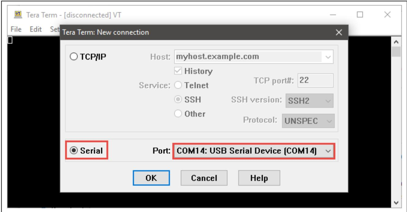
Figure 5. Selecting the Serial Port on Tera Term
