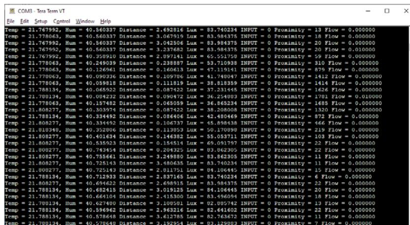
Figure 4: Measures printed on the UART port.
