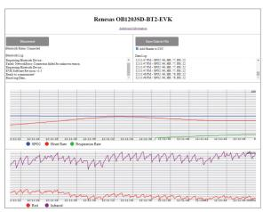
Optionally the measurements can be observed using a USB cable and SerialPlot.
