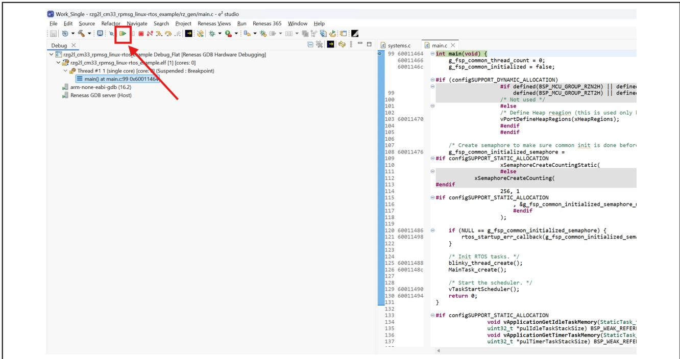
Figure 4-9. How to start to debug sample project (2)
