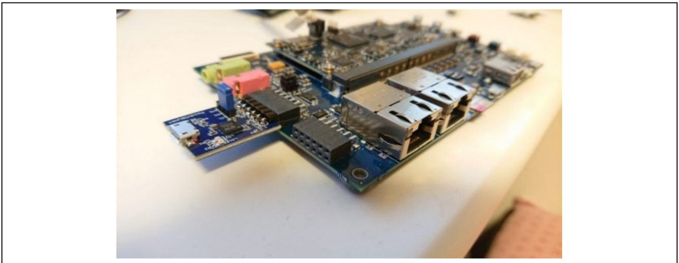
**Figure 4-1. Connection between RZ/G2L SMARC EVK and Pmod USBUART**
