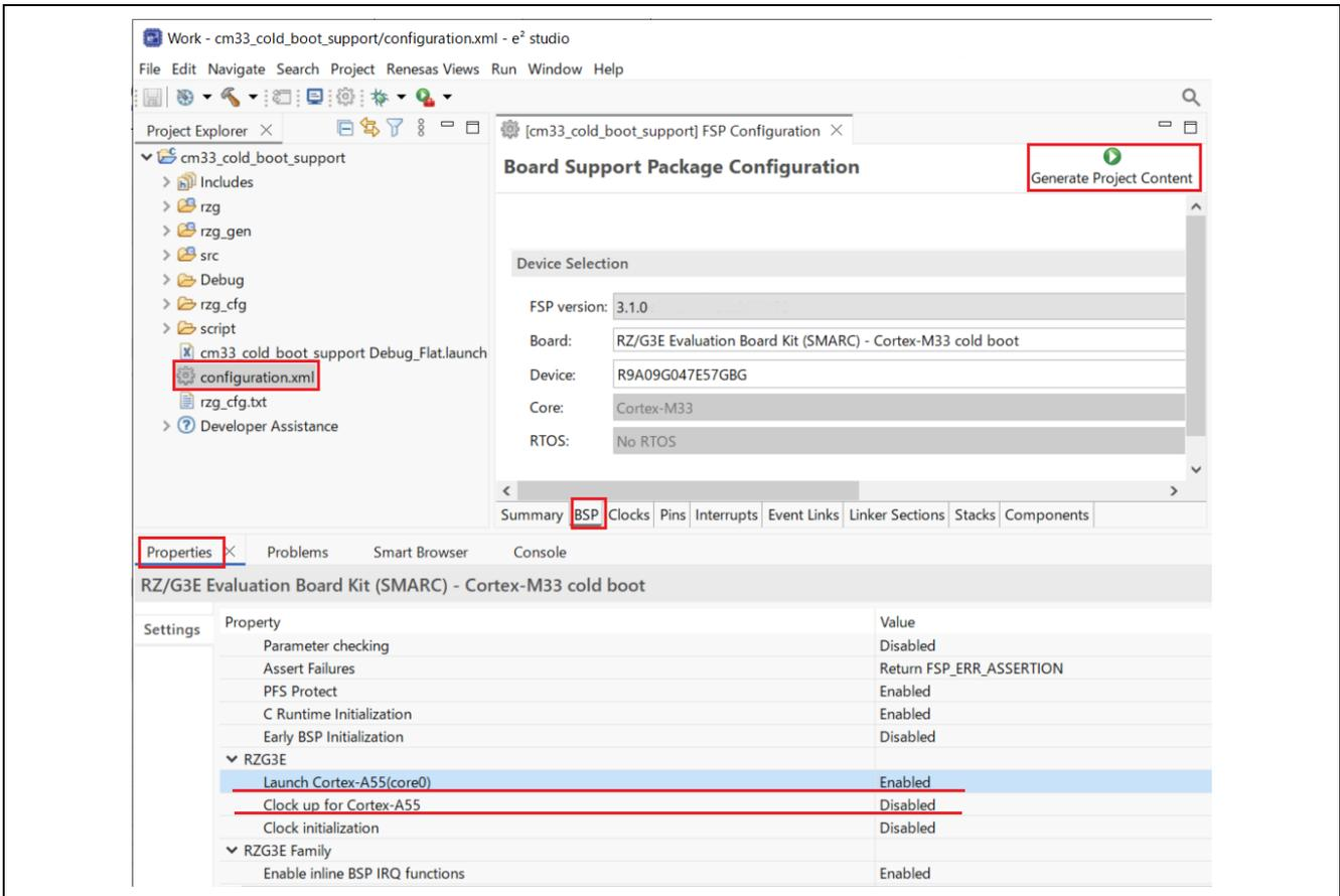
Figure 6-2. CM33 project setting for CM33 cold boot
