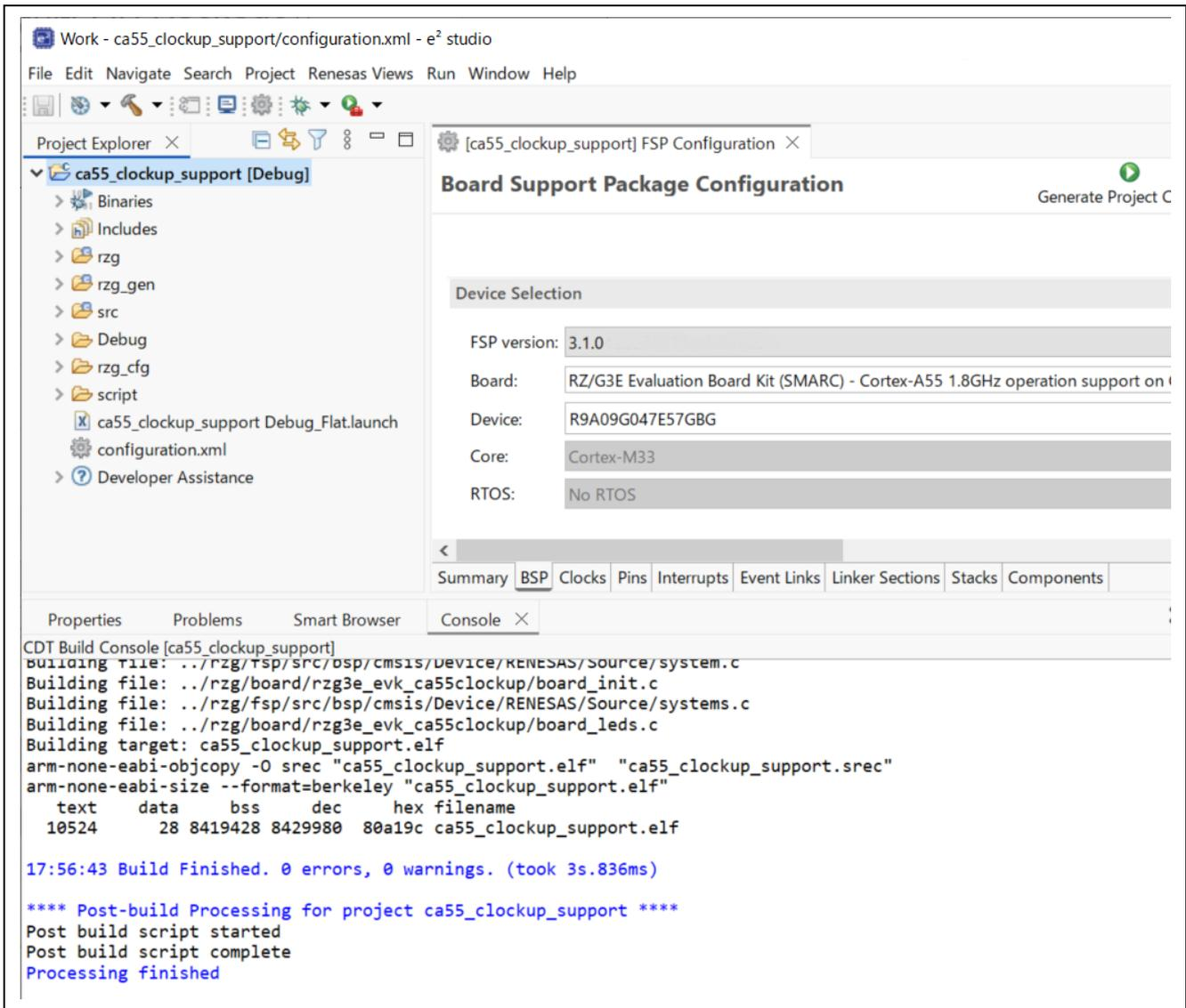
Figure 5-3. Build CM33 project for CA55 1.8GHz support
