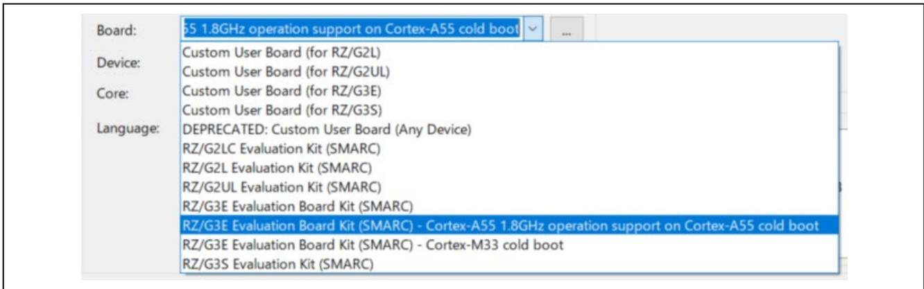
**Figure 5-1. Select board for CA55 1.8GHz operation**
