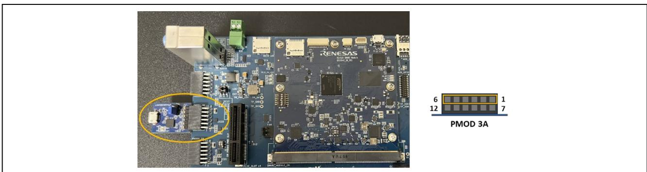
Figure 4-1. Connection between Pmod USBUART and RZ/G3S SMARC EVK
