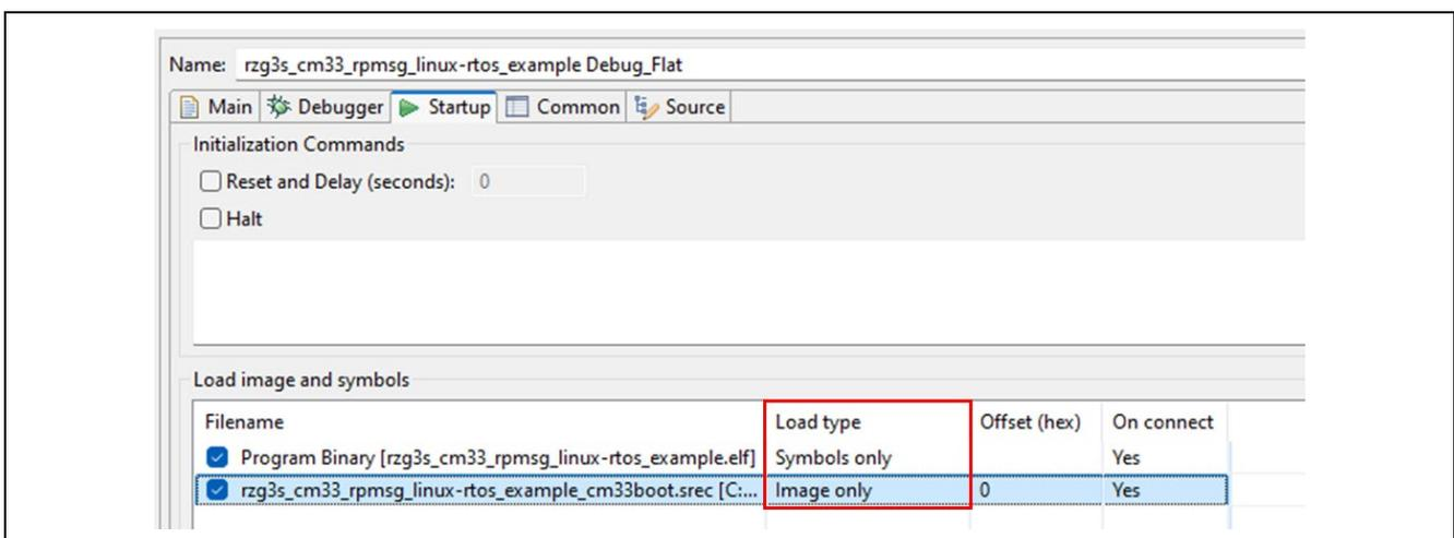
**Figure 4-13. Configuration of Load type**
