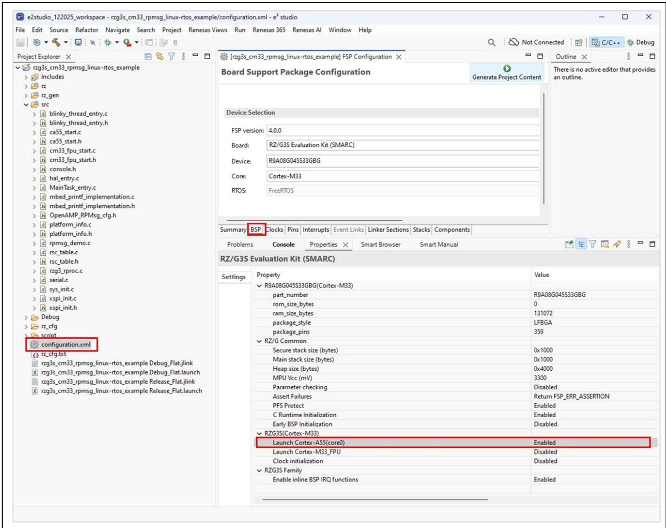
Figure 4-5. Linux boot configuration from CM33 cold boot
