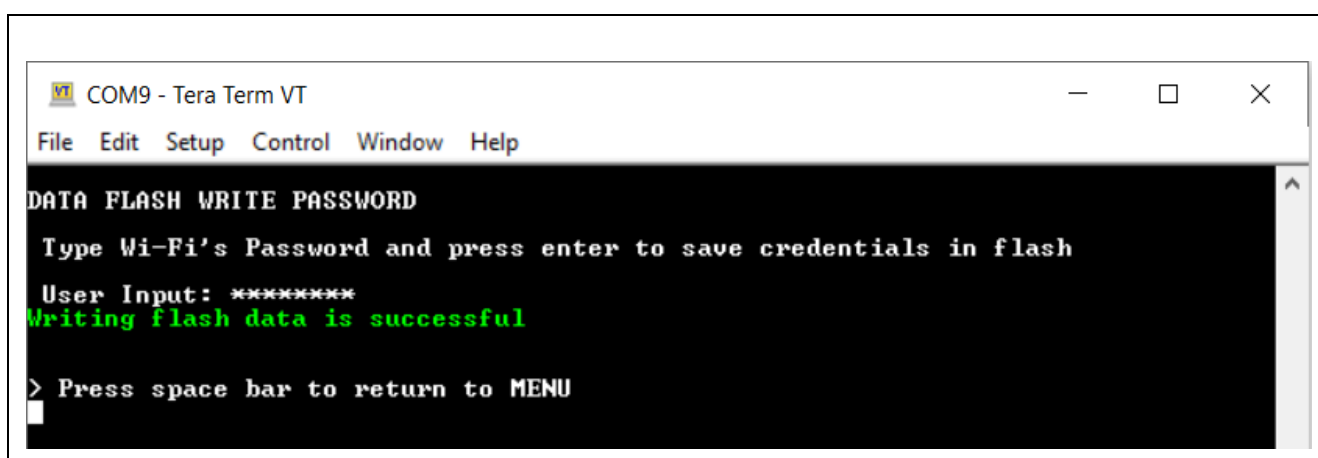
Figure 34. Storing the Wi-Fi password into the Data Flash
