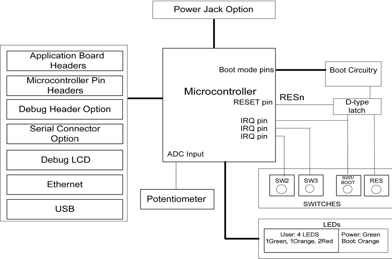
Figure 5-1: Block Diagram
