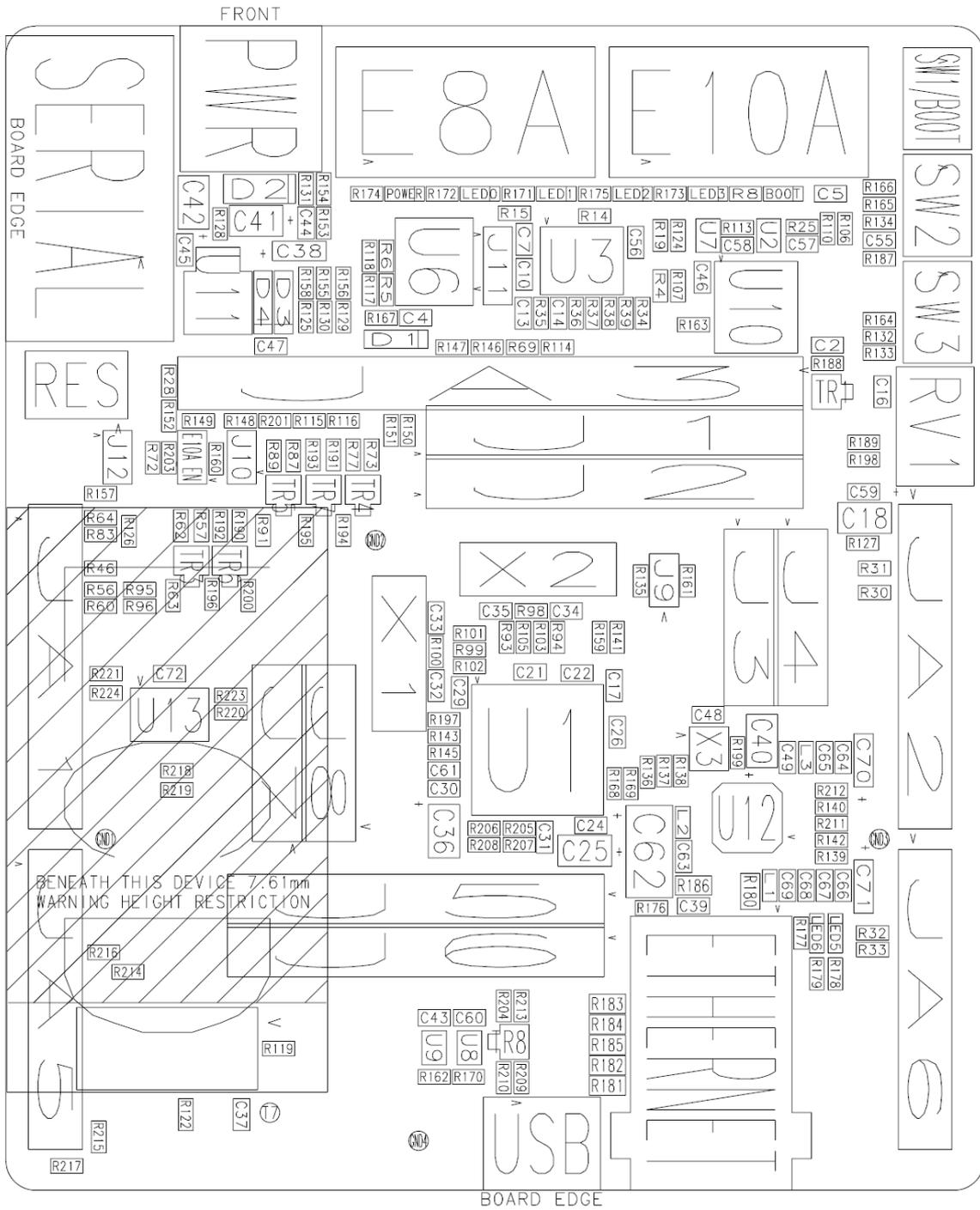
Figure 11-1: Component Placement – Front view
