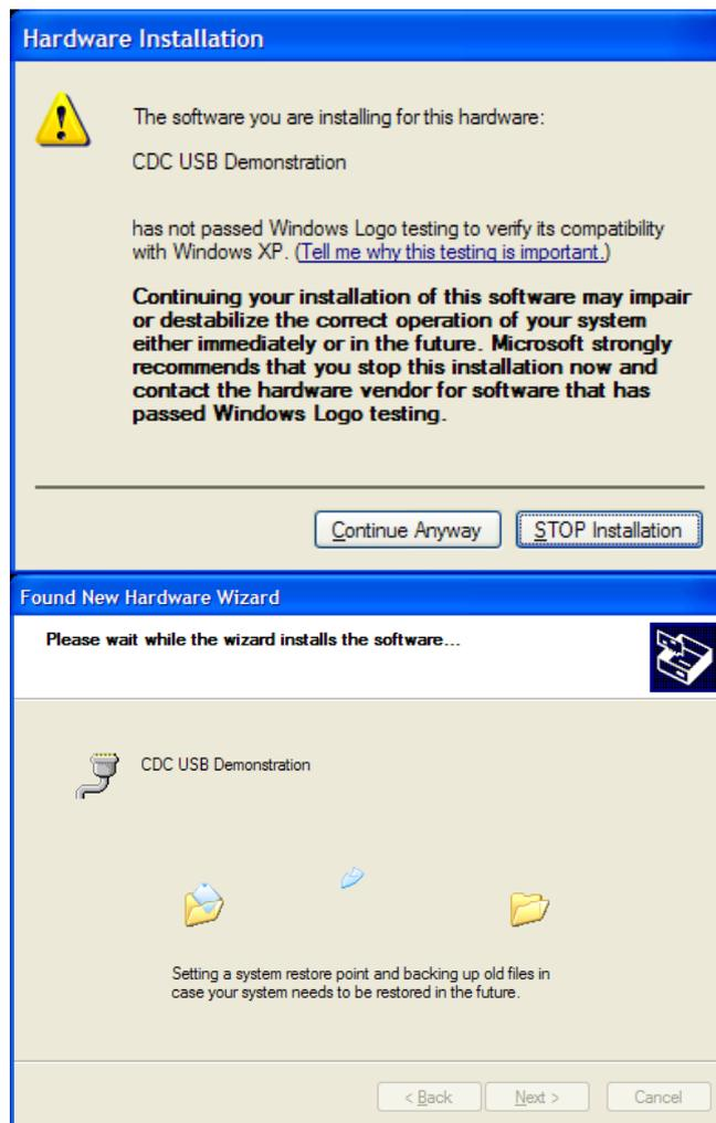
An additional COM port will become available to Windows Applications. To be able to see the port that has been allocated you can open the Windows Device Manager window. To do this, go to the start menu and select run. In the dialog displayed type "devmgmt.msc". This will open the device manager. Expand the group of serial ports and the installed ports will be listed. When the Serial Terminal program connects to this COM port\*, it will receive a repeating message from the RSK saying:
