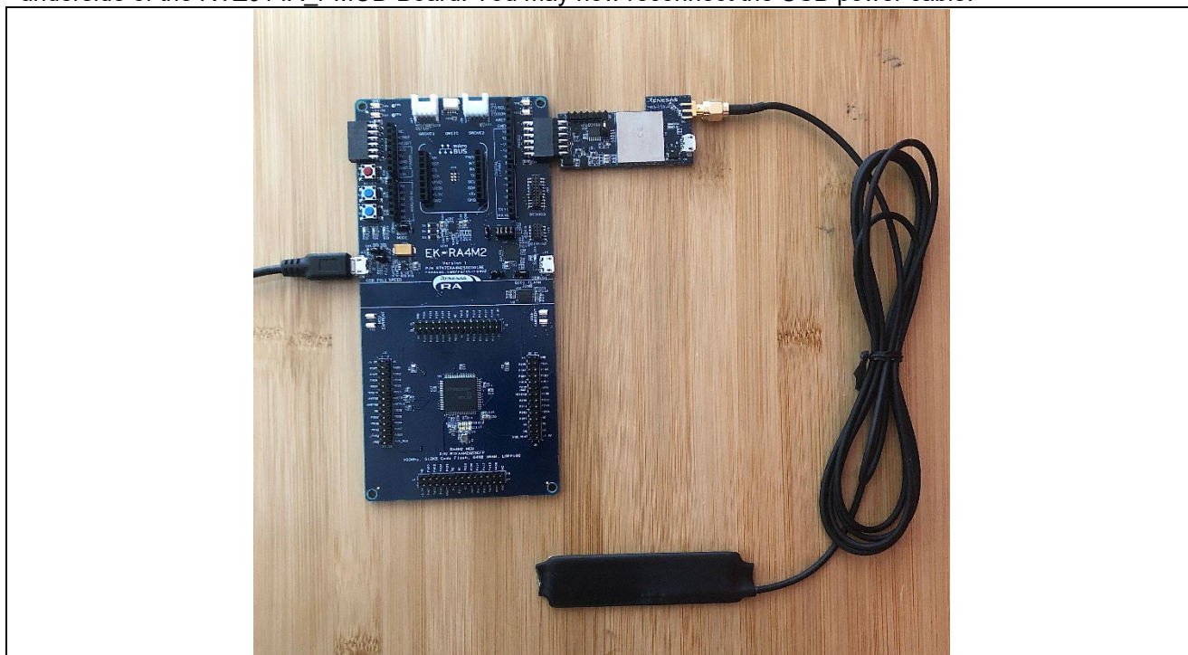
Figure 1. EK-RA4M2 Setup with RYZ014A_PMOD Module Connected
