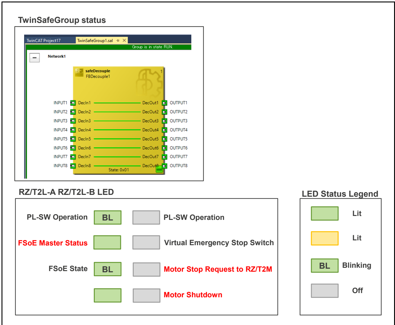
Figure 6.34. TwinSAFEGroup and RZ/T2L-A, RZ/T2L-B LEDs during Safety Signal I/O
