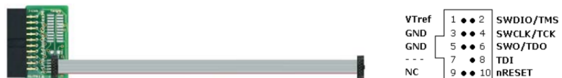
Figure 41. J-Link 9-pin Cortex-M Adapter
