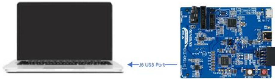
Figure 3. Connecting the VOICE-RA4E1 Board to the Host PC via USB Debug Port
