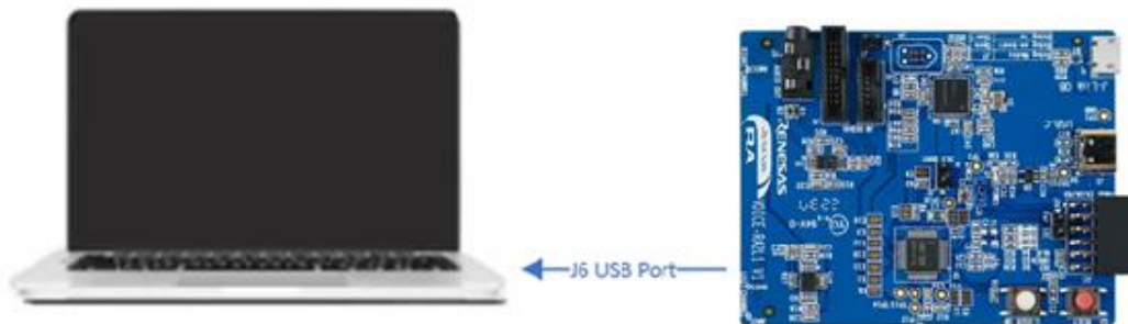
Figure 17. Connecting the VOICE-RA4E1 Board to the Host PC via USB Debug Port
