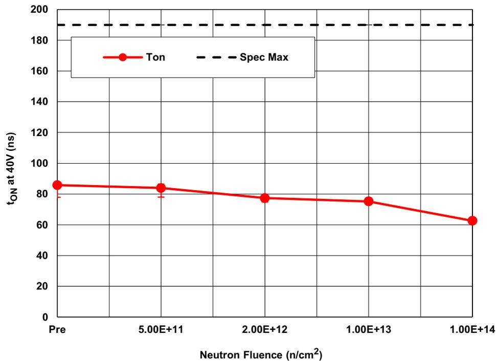
Figure 8. ISL70592SEH turn-on time at 40V ( $t_{ON}$ ), following irradiation to each neutron fluence level. The error bars represent the minimum and maximum measured values. The post-irradiation SMD limit is  $190 \mu\text{s}$  maximum.
