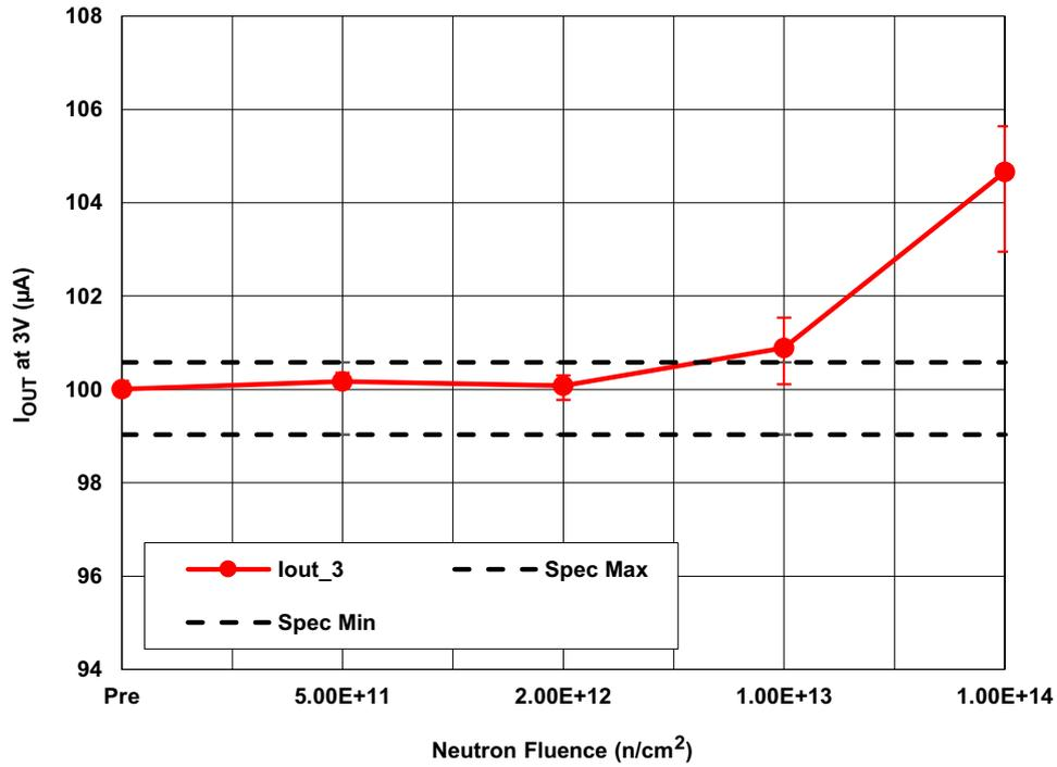
Figure 5. ISL70591SEH output current at 3V ( $I_{O3V}$ ), following irradiation to each neutron fluence level. The error bars represent the minimum and maximum measured values. The post-irradiation SMD limits are 99.03μA minimum and 100.58μA maximum.
