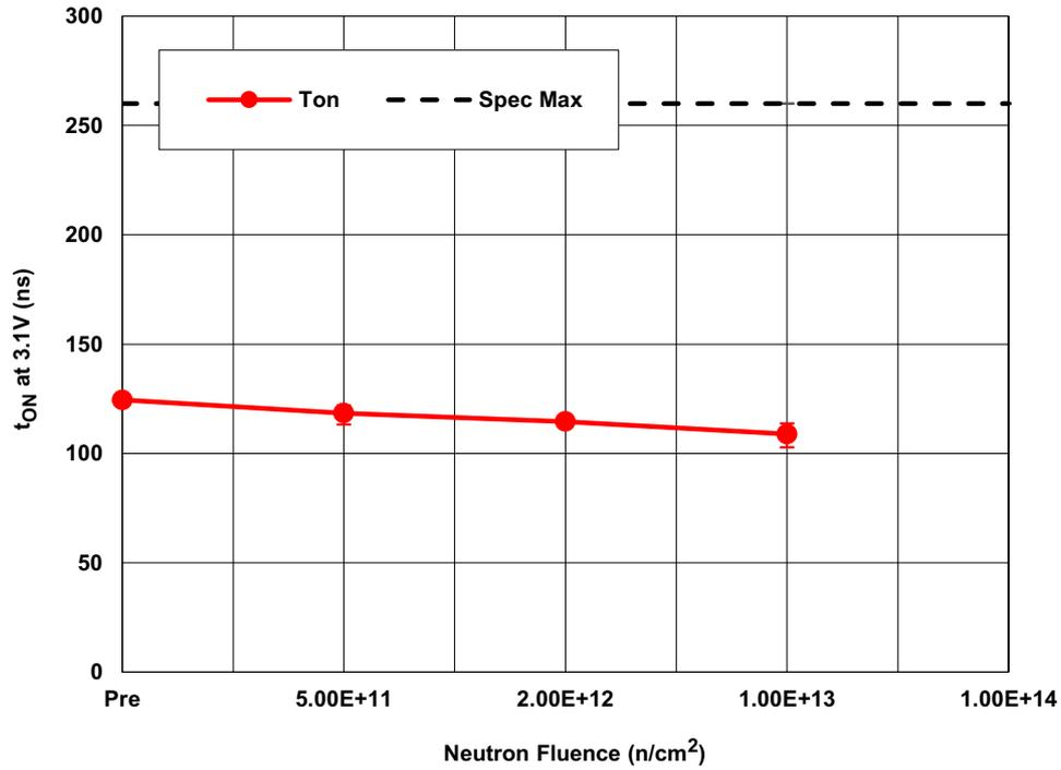
Figure 7. ISL70591SEH turn-on time at 3.1V ( $t_{ON}$ ), following irradiation to each neutron fluence level. The error bars represent the minimum and maximum measured values. The  $1 \times 10^{14} \text{ n/cm}^2$  data are not shown because they could not be accurately measured. The post-irradiation SMD limit is  $260 \mu\text{s}$  maximum.
