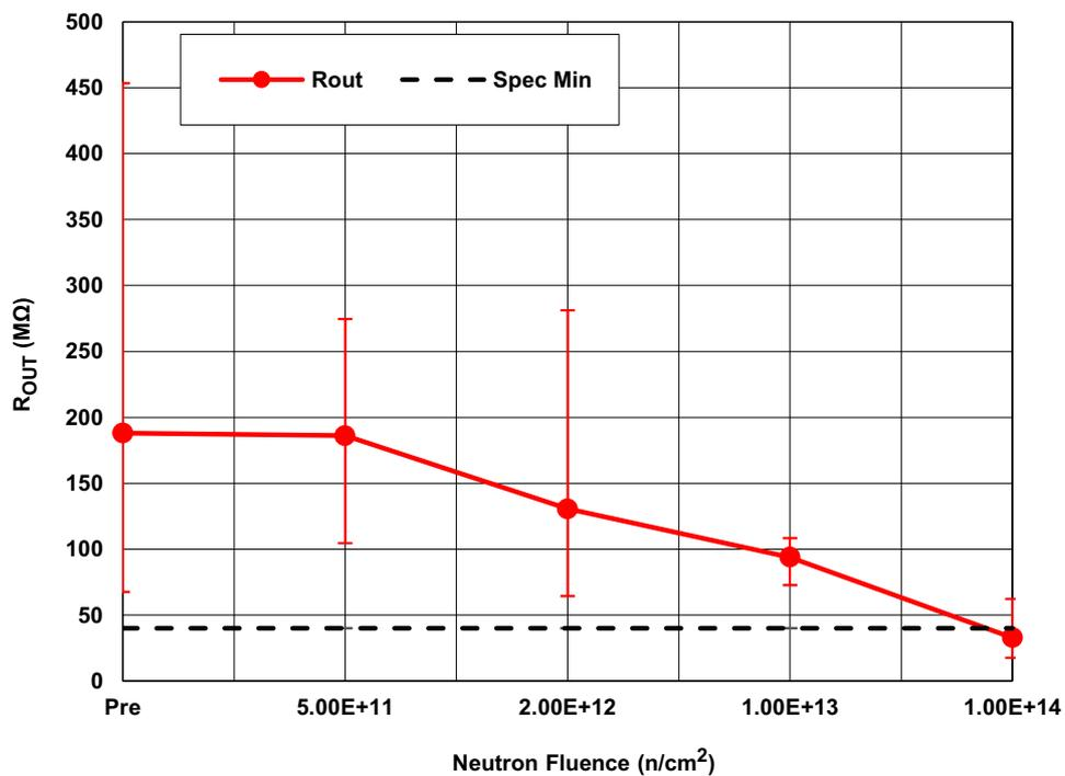
Figure 6. ISL70591SEH output impedance ( $R_{OUT}$ ), following irradiation to each neutron fluence level. The error bars represent the minimum and maximum measured values. The post-irradiation SMD limit is 40MΩ minimum.
