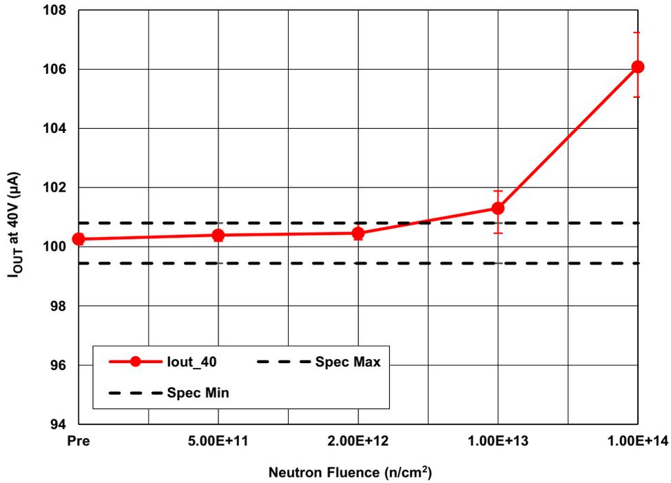
Figure 1. ISL70591SEH output current at 40V ( $I_{O40V}$ ), following irradiation to each neutron fluence level. The error bars represent the minimum and maximum measured values. The post-irradiation SMD limits are 99.44μA minimum and 100.80μA maximum.
