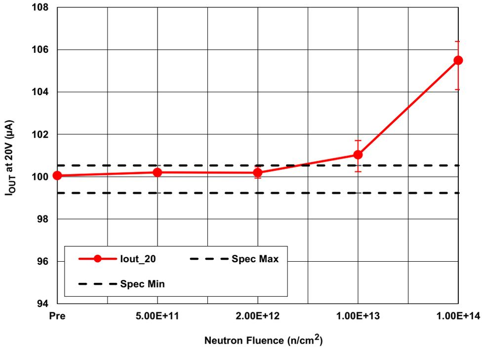
Figure 3. ISL70591SEH output current at 20V ( $I_{O20V}$ ), following irradiation to each neutron fluence level. The error bars represent the minimum and maximum measured values. The post-irradiation SMD limits are 99.23μA minimum and 100.53μA maximum.
