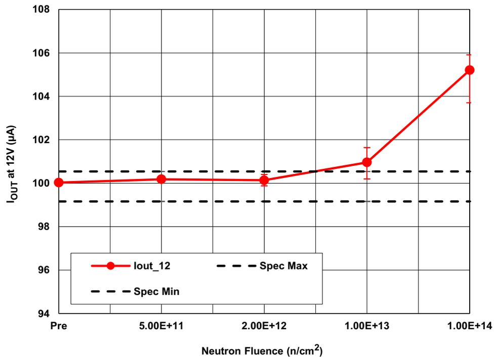
Figure 4. ISL70591SEH output current at 12V ( $I_{O12V}$ ), following irradiation to each neutron fluence level. The error bars represent the minimum and maximum measured values. The post-irradiation SMD limits are 99.16μA minimum and 100.54μA maximum.
