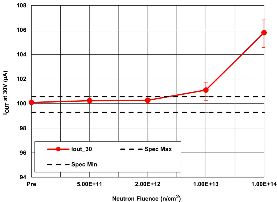
Figure 2. ISL70591SEH output current at 30V ( $I_{O30V}$ ), following irradiation to each neutron fluence level. The error bars represent the minimum and maximum measured values. The post-irradiation SMD limits are 99.29μA minimum and 100.57μA maximum.
