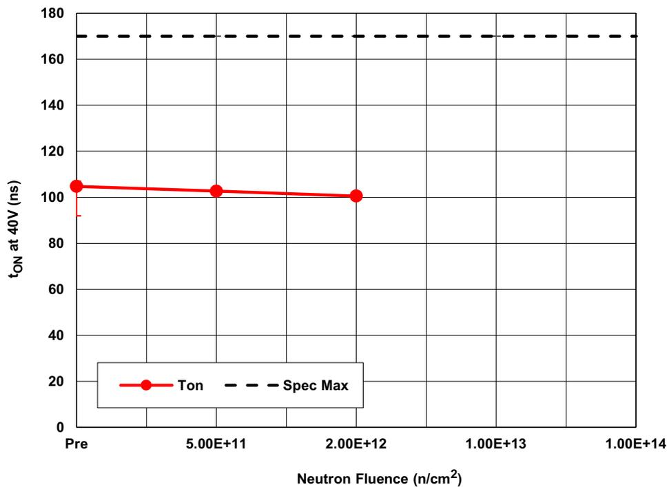
Figure 8. ISL70592SEH turn-on time at 40V ( $t_{ON}$ ), following irradiation to each neutron fluence level. The error bars represent the minimum and maximum measured values. The  $1 \times 10^{13} \text{ n/cm}^2$  and  $1 \times 10^{14} \text{ n/cm}^2$  data are not shown because they could not be accurately measured. The post-irradiation SMD limit is  $170 \mu\text{s}$  maximum.
