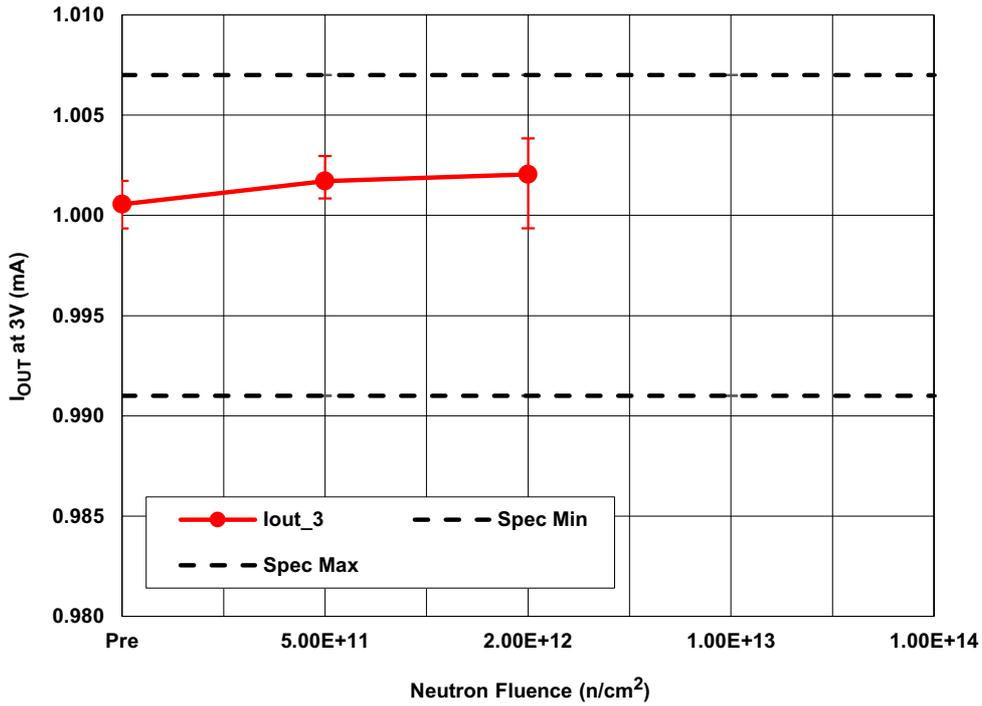
Figure 5. ISL70592SEH output current at 3V ( $I_{O3V}$ ), following irradiation to each neutron fluence level. The error bars represent the minimum and maximum measured values. The  $1 \times 10^{13} \text{ n/cm}^2$  and  $1 \times 10^{14} \text{ n/cm}^2$  data are not shown because they could not be accurately measured. The post-irradiation SMD limits are 0.9910mA minimum and 1.0070mA maximum.
