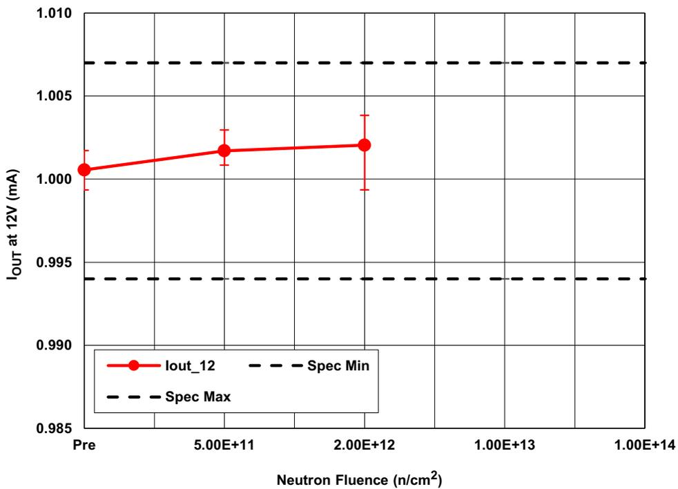
Figure 4. ISL70592SEH output current at 12V ( $I_{O12V}$ ), following irradiation to each neutron fluence level. The error bars represent the minimum and maximum measured values. The  $1 \times 10^{13} \text{ n/cm}^2$  and  $1 \times 10^{14} \text{ n/cm}^2$  data are not shown because they could not be accurately measured. The post-irradiation SMD limits are 0.9930mA minimum and 1.0070mA maximum.
