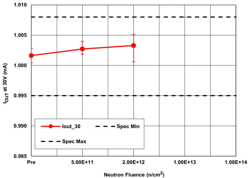
Figure 2. ISL70592SEH output current at 30V ( $I_{O30V}$ ), following irradiation to each neutron fluence level. The error bars represent the minimum and maximum measured values. The  $1 \times 10^{13} \text{ n/cm}^2$  and  $1 \times 10^{14} \text{ n/cm}^2$  data are not shown because they could not be accurately measured. The post-irradiation SMD limits are 0.9950mA minimum and 1.0080mA maximum.
