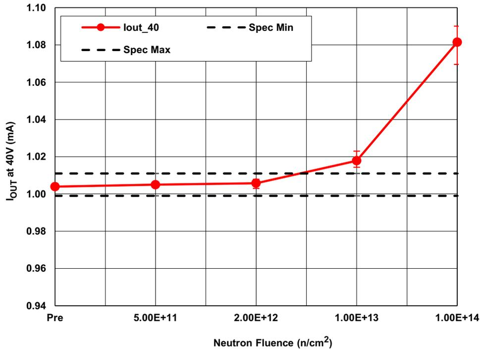
Figure 1. ISL70592SEH output current at 40V ( $I_{O40V}$ ), following irradiation to each neutron fluence level. The error bars represent the minimum and maximum measured values. The post-irradiation SMD limits are 0.9990mA minimum and 1.0110mA maximum.
