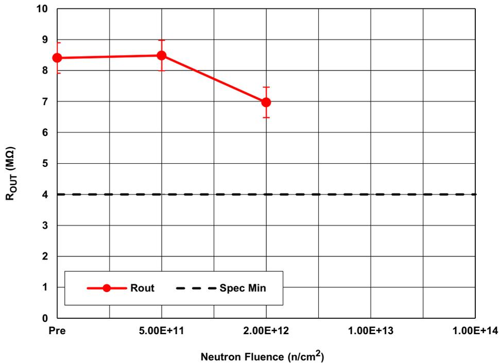
Figure 6. ISL70592SEH output impedance ( $R_{OUT}$ ), following irradiation to each neutron fluence level. The error bars represent the minimum and maximum measured values. The  $1 \times 10^{13} \text{ n/cm}^2$  and  $1 \times 10^{14} \text{ n/cm}^2$  data are not shown because they could not be accurately measured. The post-irradiation SMD limit is 4MΩ minimum.
