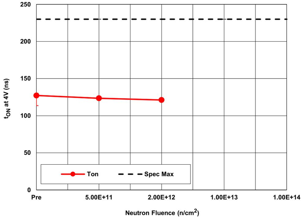
Figure 7. ISL70592SEH turn-on time at 4V ( $t_{ON}$ ), following irradiation to each neutron fluence level. The error bars represent the minimum and maximum measured values. The  $1 \times 10^{13} \text{ n/cm}^2$  and  $1 \times 10^{14} \text{ n/cm}^2$  data are not shown because they could not be accurately measured. The post-irradiation SMD limit is  $230 \mu\text{s}$  maximum.
