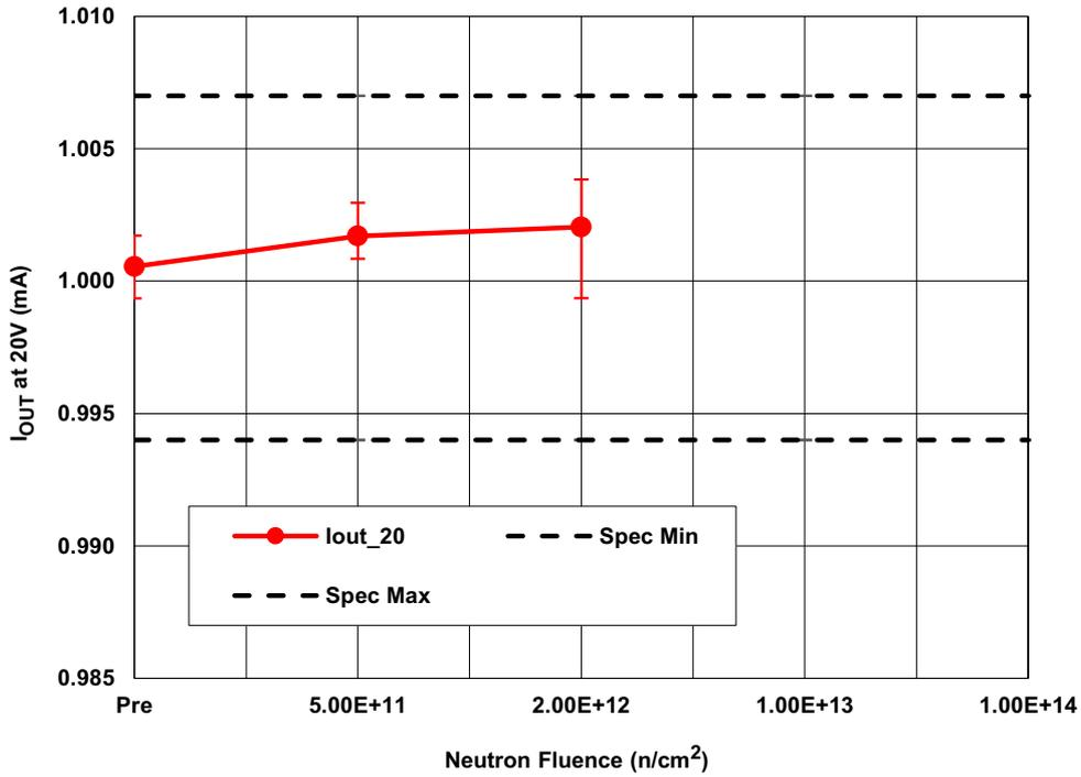
Figure 3. ISL70592SEH output current at 20V ( $I_{O20V}$ ), following irradiation to each neutron fluence level. The error bars represent the minimum and maximum measured values. The  $1 \times 10^{13} \text{ n/cm}^2$  and  $1 \times 10^{14} \text{ n/cm}^2$  data are not shown because they could not be accurately measured. The post-irradiation SMD limits are 0.9940mA minimum and 1.0070mA maximum.
