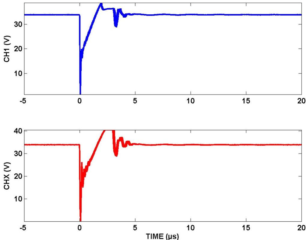
**Figure 4. Composite plot of CH1 (coincidental) and CHX (triggered at 2V) SET where both exceeded 30V deviation on the same capture. This plot is the seven events captured on DUT9 for  $86\text{MeV}\cdot\text{cm}^2/\text{mg}$  irradiation.**
