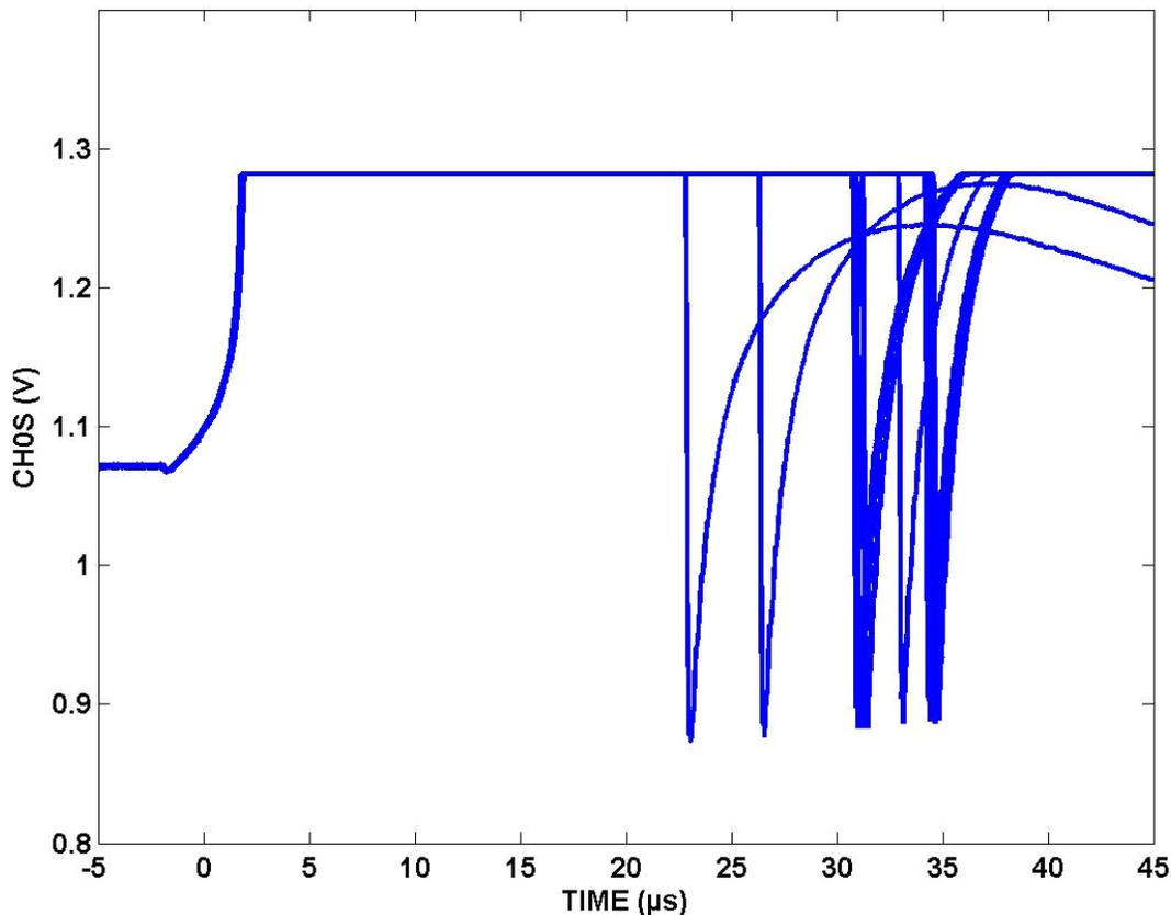
Figure 5. Composite of the 14 ON CH0 transients that exceeded 100mV for more than 1µs for DUT19 run at 20MeV·cm<sup>2</sup>/mg with V<sub>CC</sub> = 3.0V.
