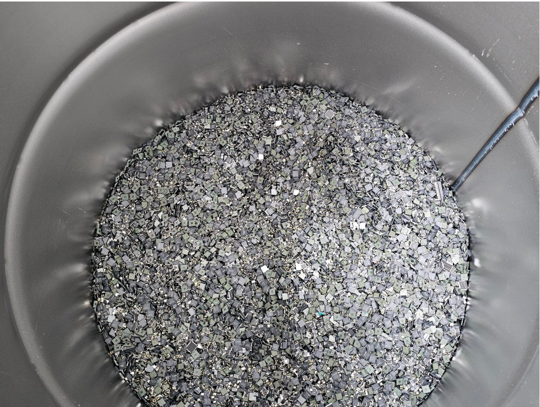
Recycling valuable materials by dismantling defective ICs accumulated over time (Bingen Site)
