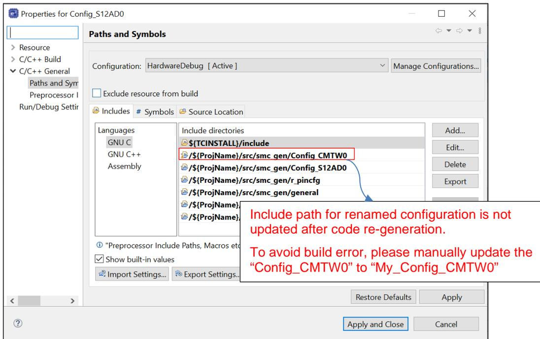
Figure 6-5 Include path setting for the “Config\_S12AD0” configuration
