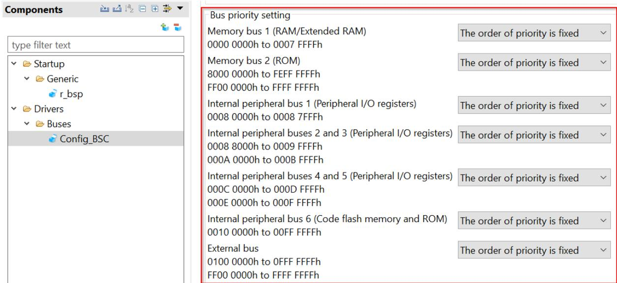
Figure 5-6 Bus priority setting with Buses component
