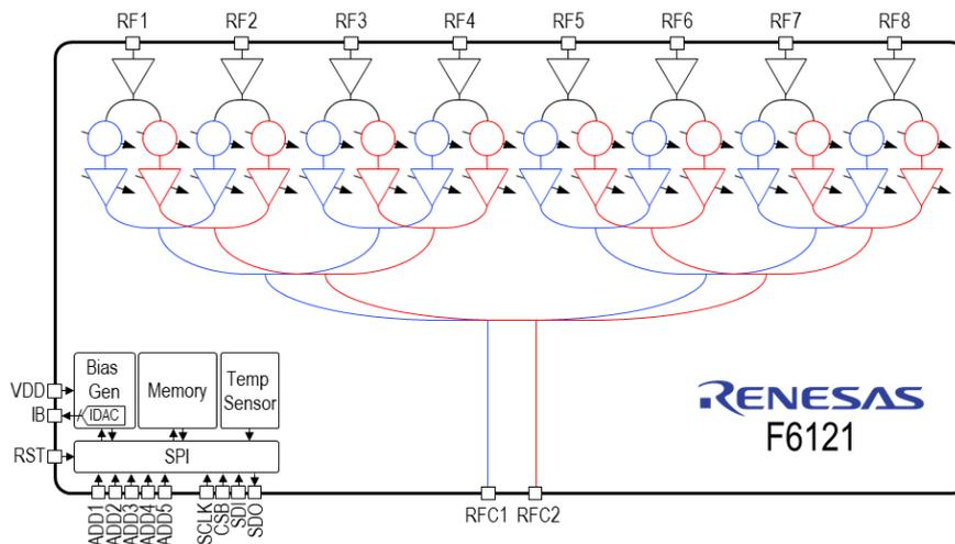
Figure 1. Block Diagram
