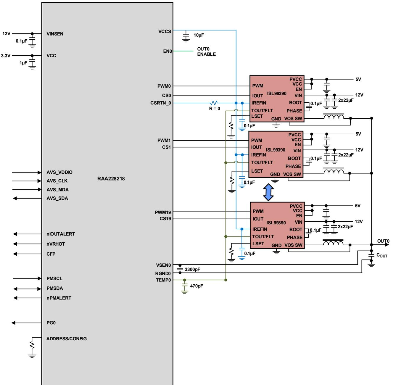
Figure 1. 20-Phase Smart Power Stage
