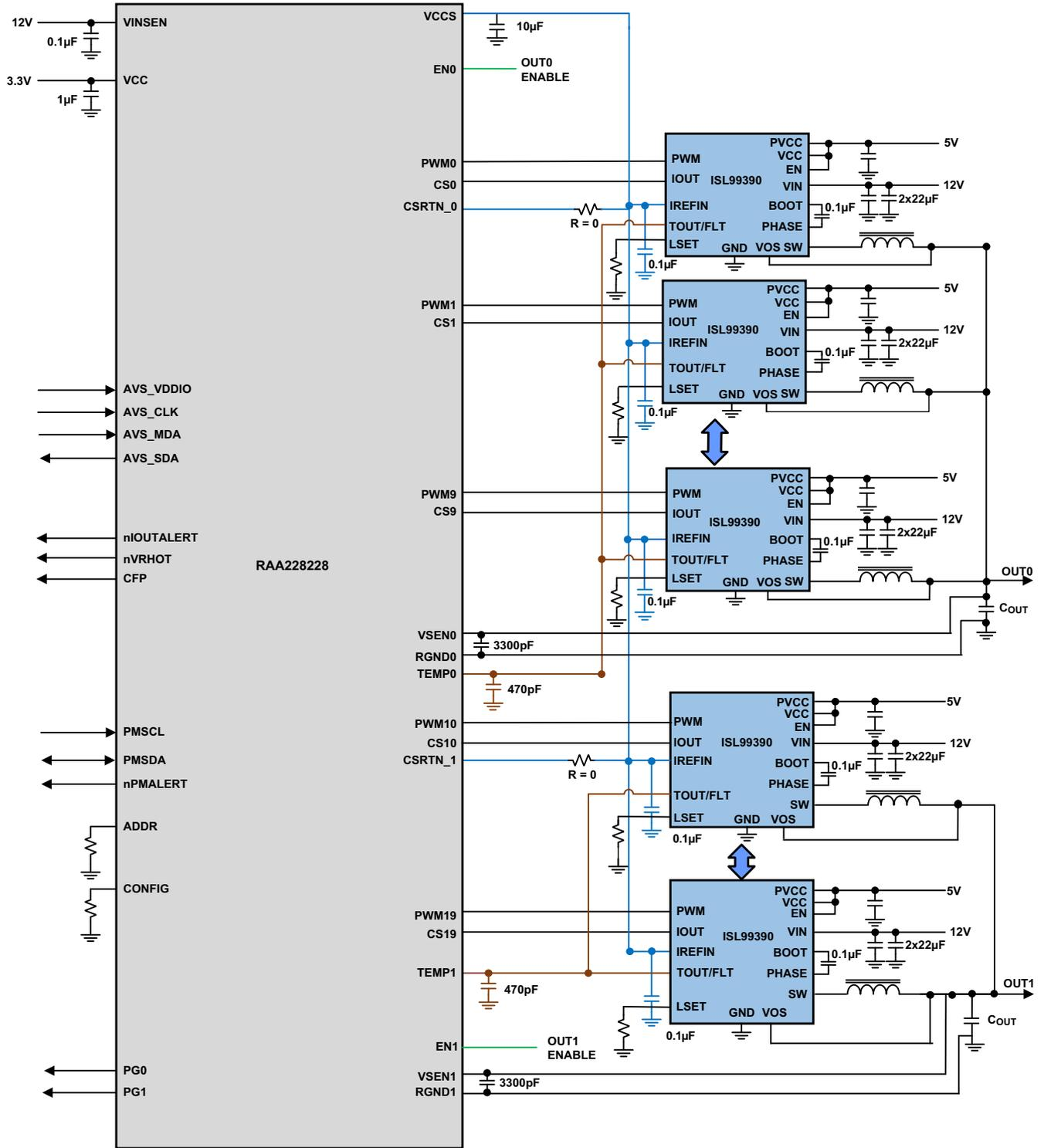
Figure 1. 10+10 Smart Power Stage
