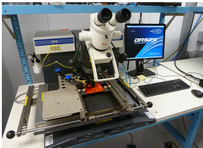
Figure 13. Rework Station with Thermal Profile Control
